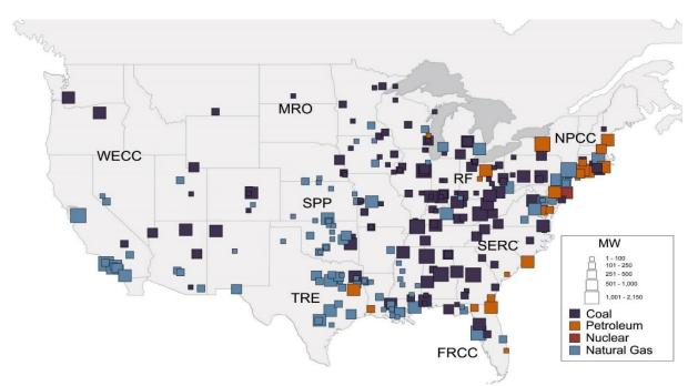
Figure 18: Generation Retirements by Fuel Type and Size<sup>26</sup>
