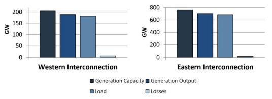
Figure 17: Generation Capacity, Load, and Losses in Eastern and Western Interconnections
