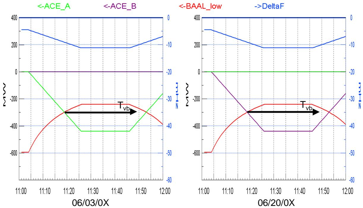
**Figure 13.** ACE trends of two BAs in two different one-hour periods when separately compared with each BA's BAAL<sub>low</sub>.
