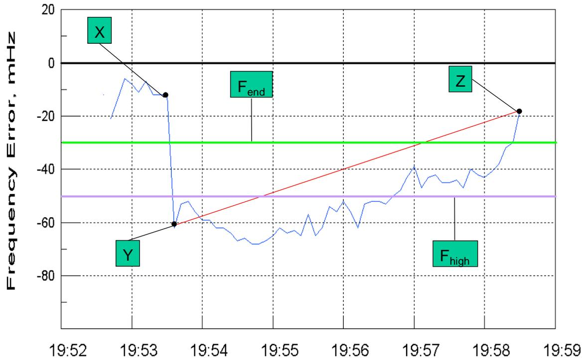
**Figure 27.** Plot of a recovery following a contingency, showing some significant points and parameters considered by the Processing phase program for this event.
