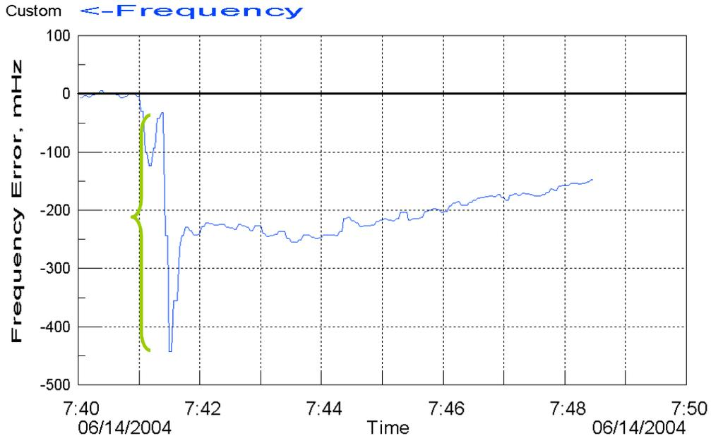
**Figure 3.** WECC frequency response to a large event. The bracket indicates the magnitude of the frequency drop considered for the estimate of P-Frequency-Response.
