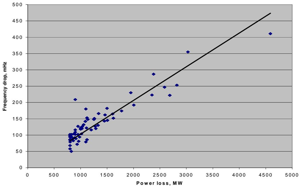
**Figure 4.** Scatter plot of the P-Frequency-Response to events recorded in WECC.
