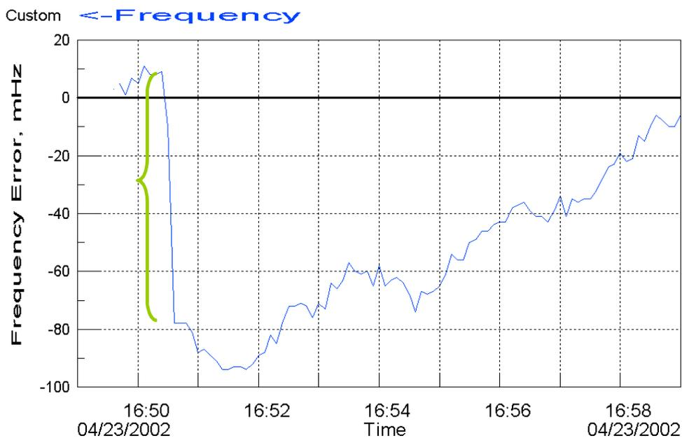
**Figure 1.** Eastern Interconnection frequency response to a large event. The bracket indicates the magnitude of the frequency drop considered for the estimate of P-Frequency-Response.
