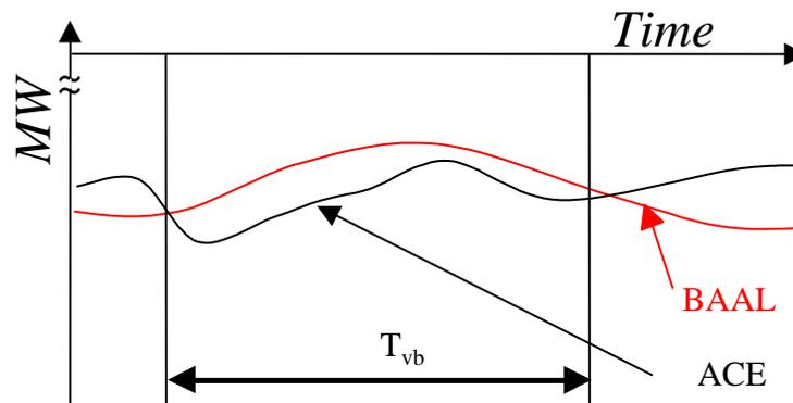
**Figure 10.** Example scenario of a BA failing BAAL measure.
