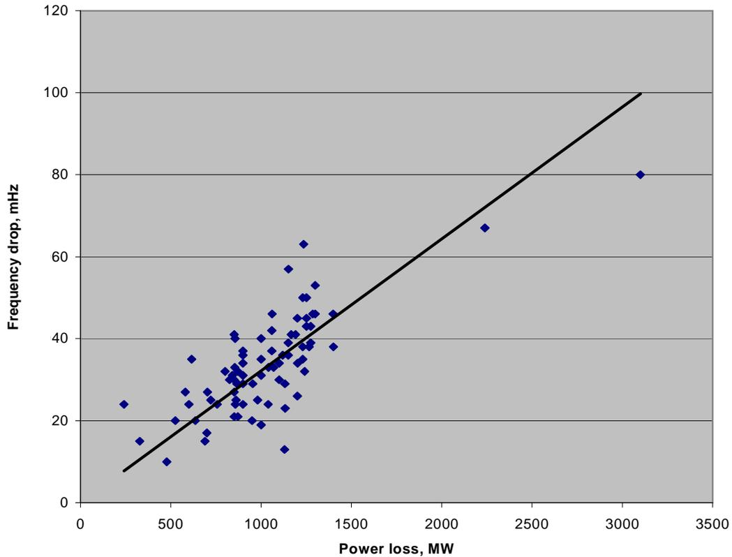
**Figure 2.** Scatter plot of the P-Frequency-Response to events recorded in the Eastern Interconnection.
