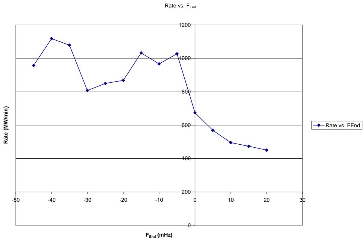
**Figure 28.** Plot of recovery rate vs.  $F_{end}$  for the Eastern Interconnection.
