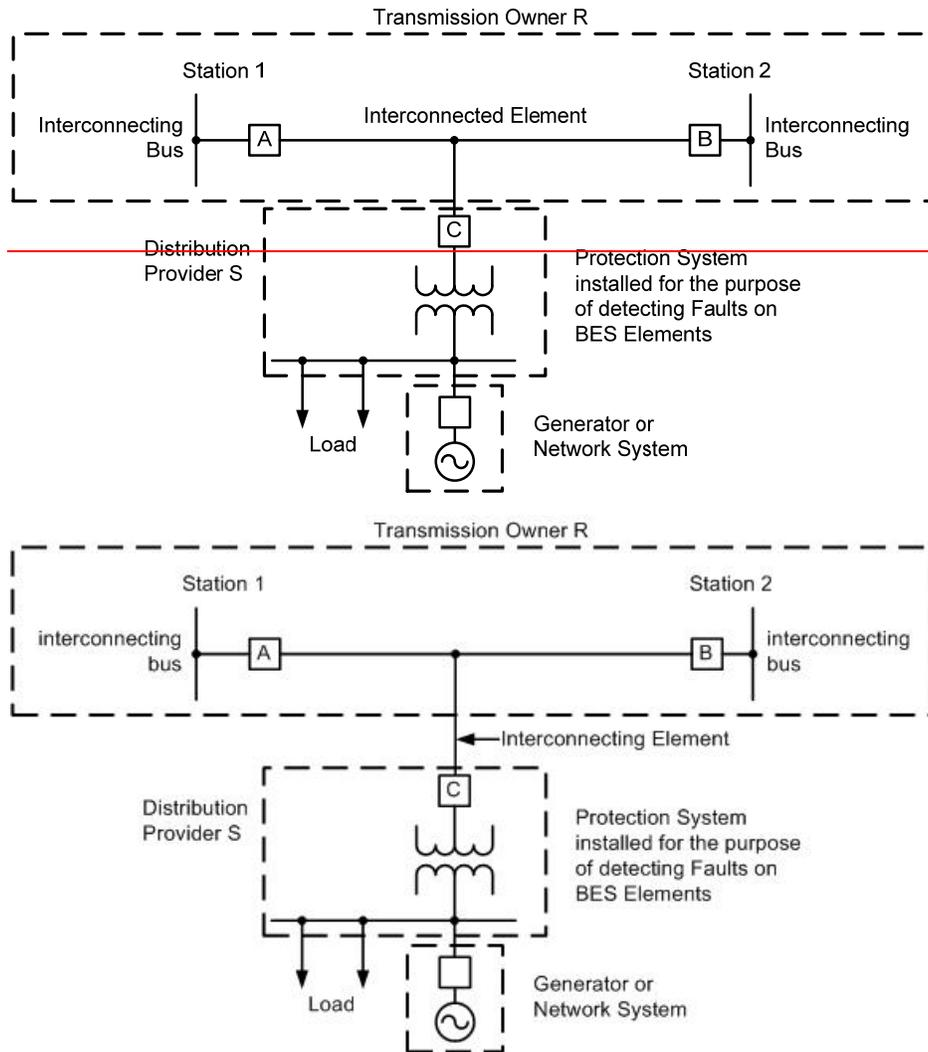
In Figure 3 above, the ~~Interconnected~~Interconnecting Element between the Transmission Owner and the Distribution Provider is the transmission line (or tap) between the Distribution Provider's Breaker C and the point of connection to the line between the Transmission Owner's Breakers A and B. Therefore, the applicable Protection Systems per this standard are those at Breakers A, B and C.
