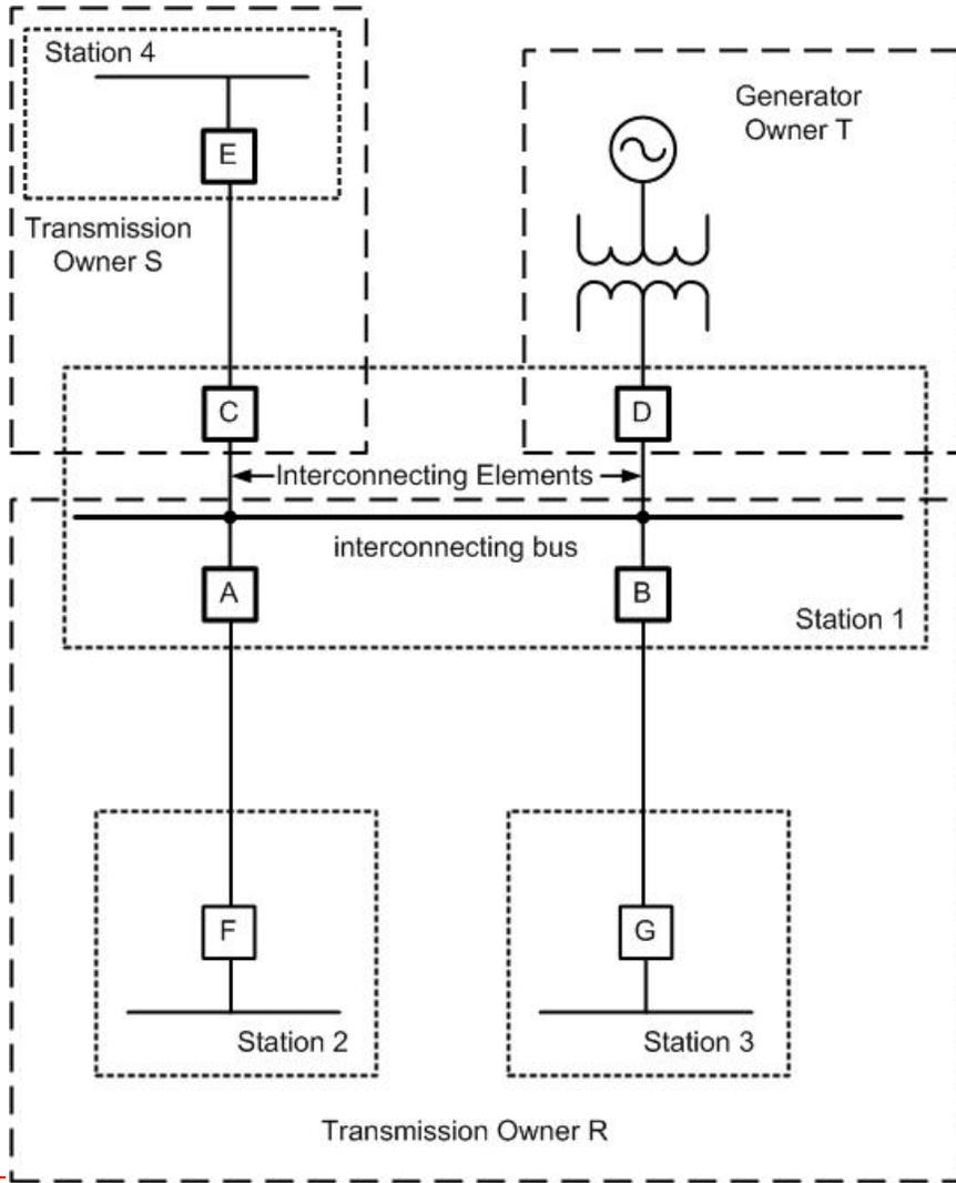
In Figure 5 above, illustrates the Interconnecting Element Interconnecting Elements between the Transmission Owners R and S and Generator Owner T is the common Transmission bus. In this example, Transmission Owner S and Generator Owner T are not directly interconnecting to each other at Station 1. All direct interconnections are between Owner R and each of the other Owners connected to the common bus at Station 1.
