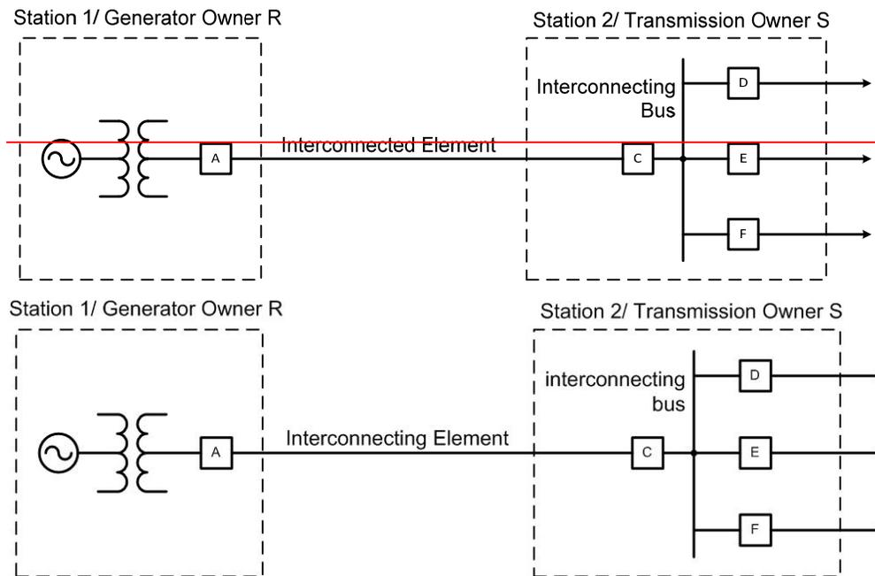
In Figure 2 above, the ~~Interconnected~~Interconnecting Element between the Transmission Owner and the Generator Owner is the transmission line or bus between Breakers A and C.
