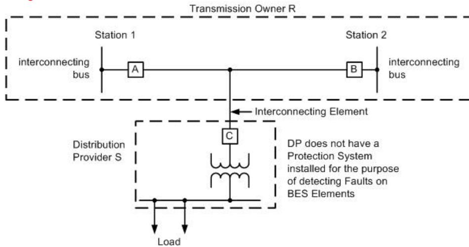
The configuration above, ~~the Interconnected Element between the Transmission Owner and~~ is an example excluded from this standard because the Distribution Provider ~~is the transmission line or tap between the line and Breaker C.~~
