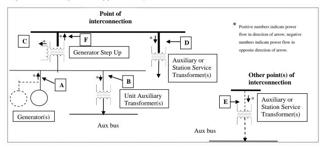
Simplified one-line diagram showing plant auxiliary Load connections and verification data:
