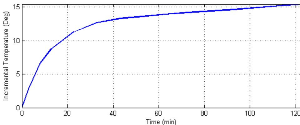
**Figure 7: Thermal Step Response to a 5 A/phase dc Step [3]
