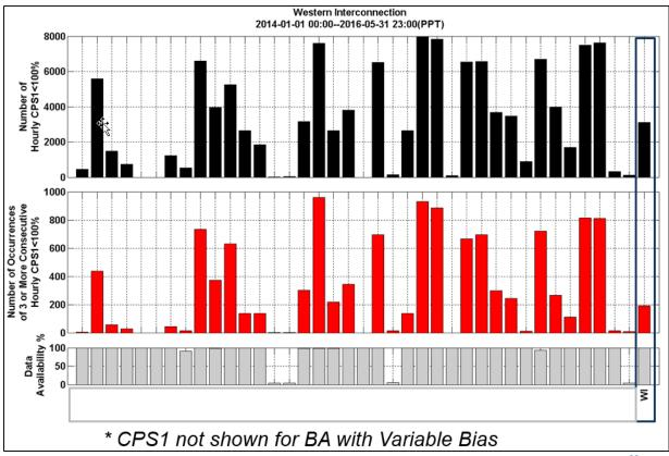
Figure 3.14: Western Interconnection—CPS1 exceedance counts per BA on an hourly basis<sup>39</sup>
