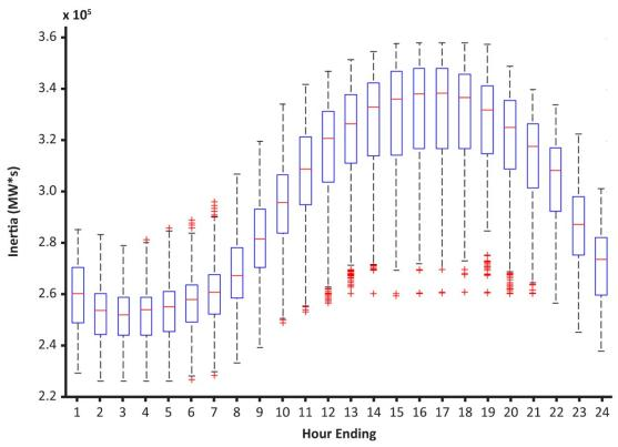
Figure 3.3: ERCOT Inertia by Hour of Day (June 1–July 15 2016)
