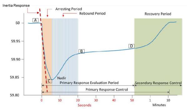
Figure 3.1: Typical Frequency Excursion and Recovery
