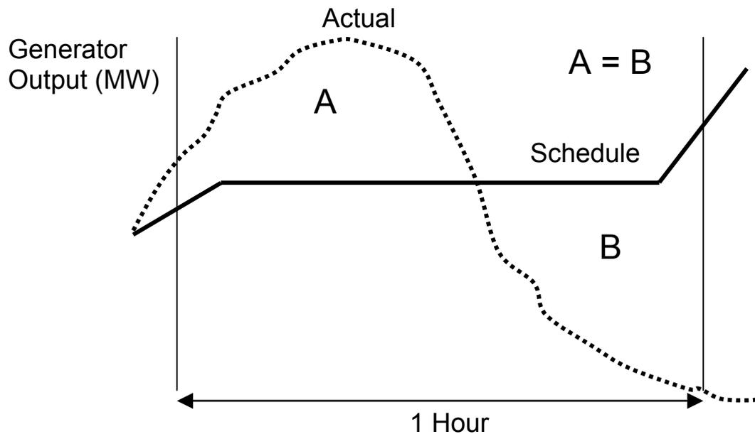
Figure 1 – Clock Hour Integrated Energy Inadequate to Measure Schedule Following
