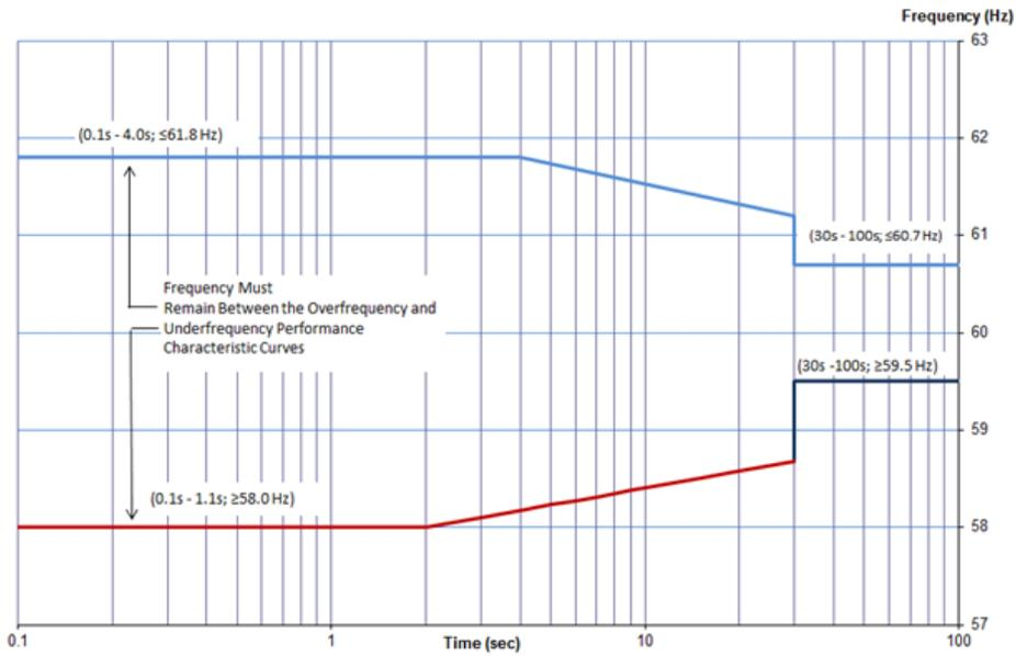
PRC-006-NPCC-2 – Automatic Underfrequency Load Shedding
