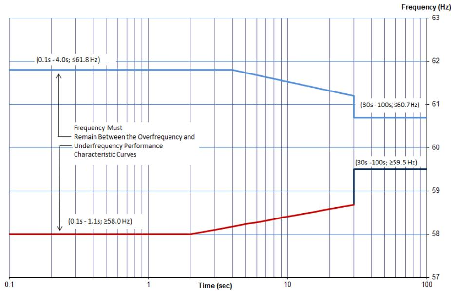
PRC-006-NPCC-2 – Automatic Underfrequency Load Shedding
