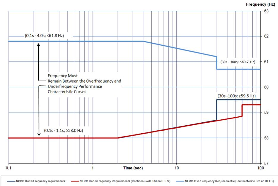
PRC-006-NPCC-2 – Automatic Underfrequency Load Shedding
