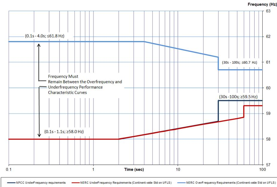
PRC-006-NPCC-2 – Automatic Underfrequency Load Shedding
