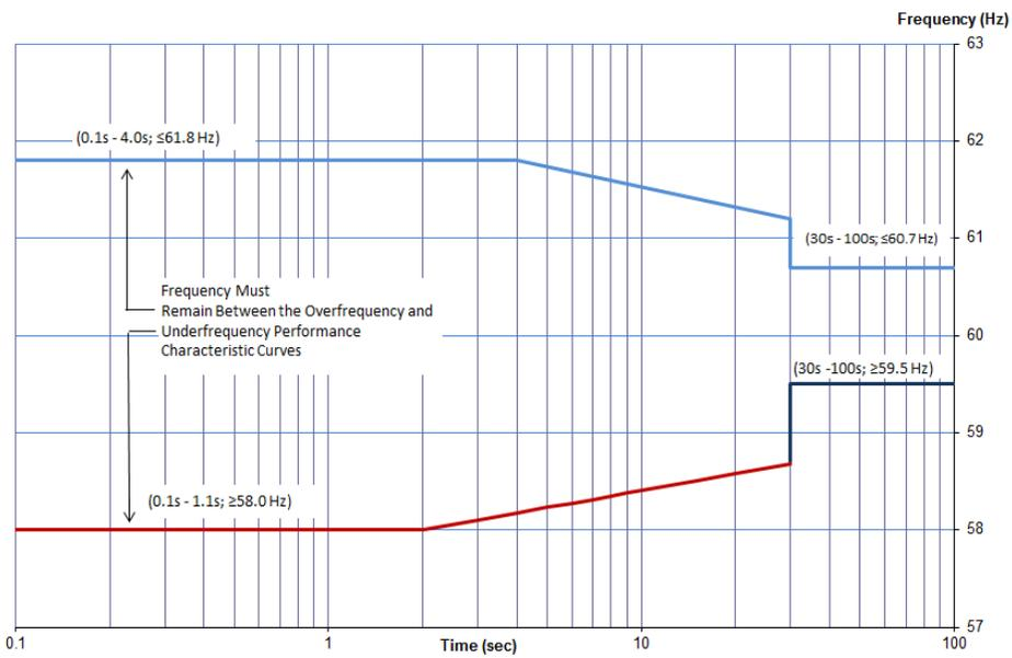
PRC-006-NPCC-2 – Automatic Underfrequency Load Shedding
