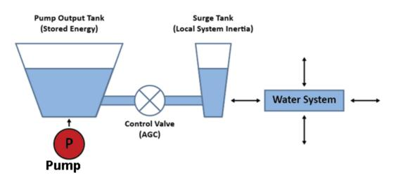
Figure 1.4: Generator | Pump Analogy
