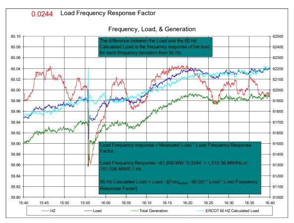
Figure 2.5: Observing Frequency Response of Load
