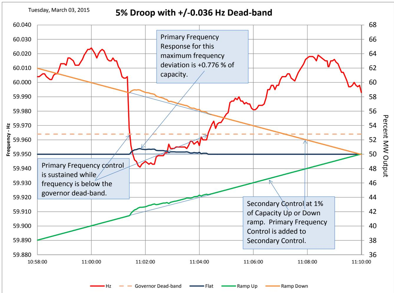
**Example of Properly Coordinated Primary Frequency Control while ramping up or down via local or remote control or while operating at a fixed output.**
