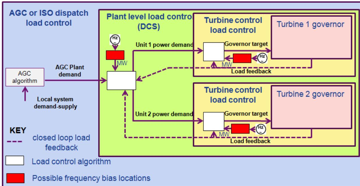
**Figure 1: Typical High Level System**
