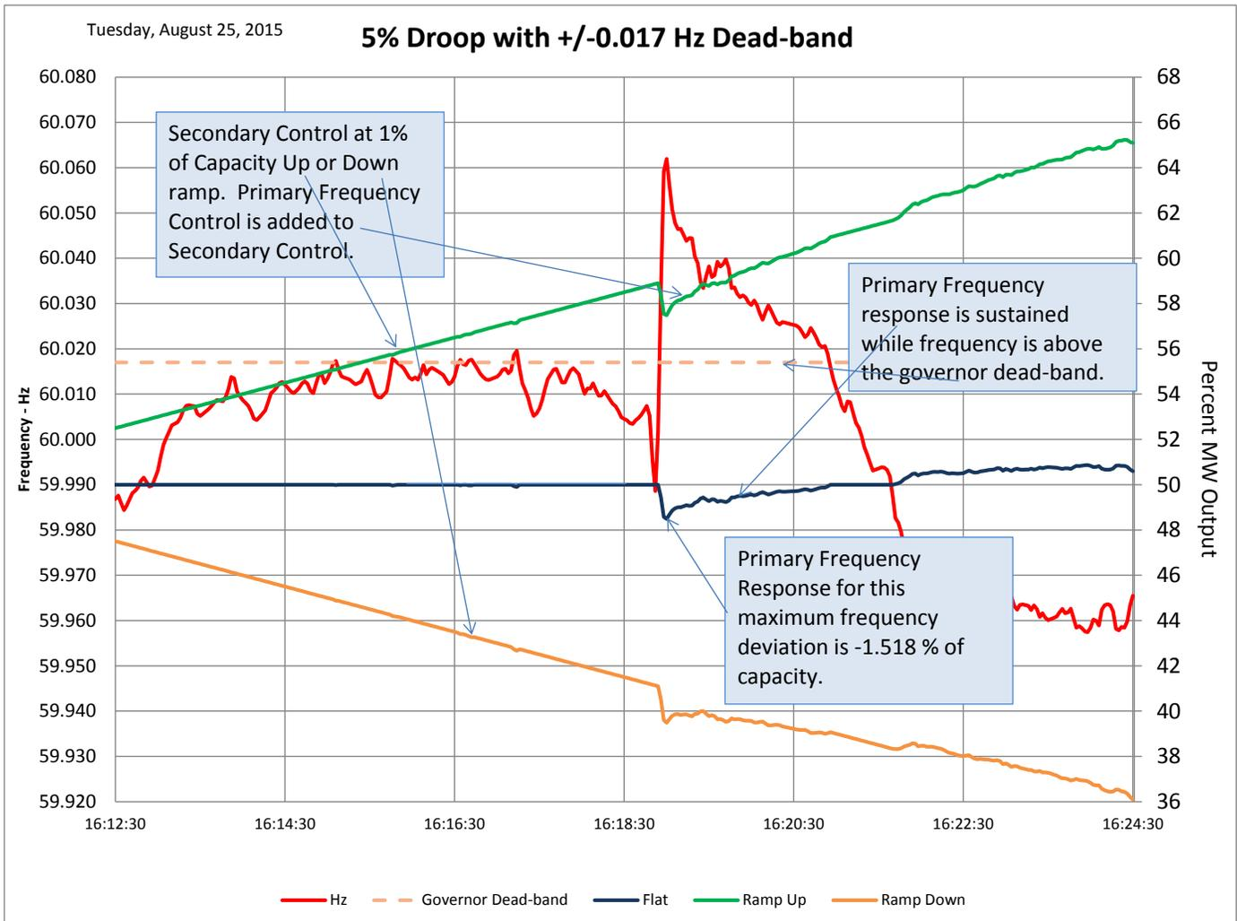
**Example of Properly Coordinated Primary Frequency Control while ramping up or down via local or remote control or while operating at a fixed output in the graph below - High Frequency excursion with a lower deadband**
