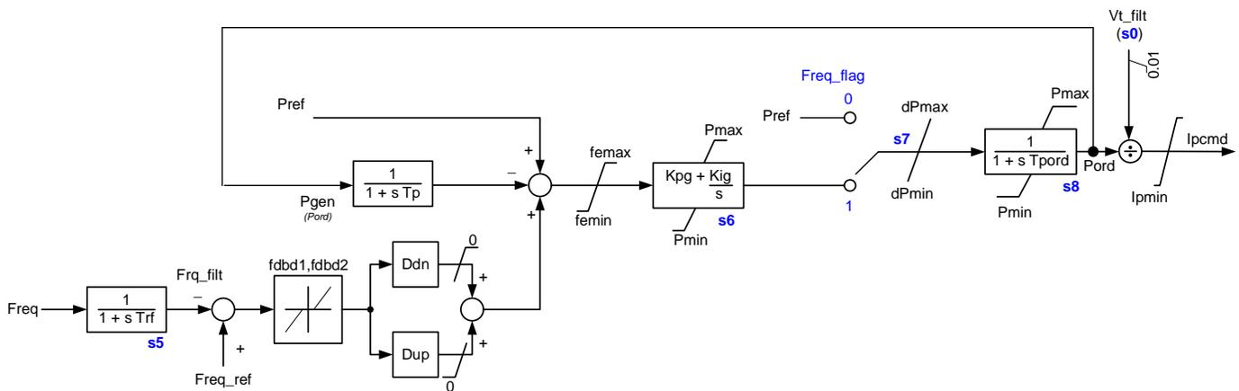
**Figure 2: *DER\_A* Active Power-Frequency Controls**
