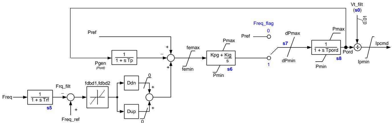
**Figure 2: *DER\_A* Active Power-Frequency Controls**
