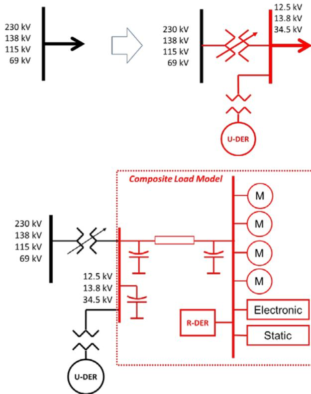
Figure 1: Representation of U-DER and R-DER
