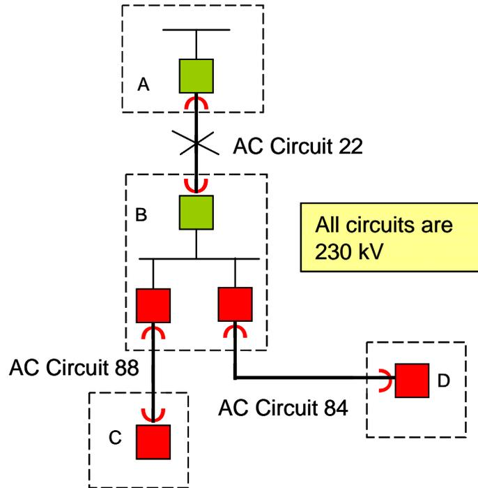
An exception that an Element be “connected at all its terminals” to be considered in an In-Service State is provided for a multi-terminal AC Circuit with a Transformer on one terminal that shares a breaker with the circuit.
