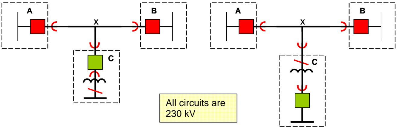
In both figures, the AC Circuit is bounded by AC Substations “A,” “B,” and “C” as indicated by the red arcs. Each Transformer’s boundaries are the red disconnect switch and the red arc before the breaker. Note that the Transformer in either figure may *or* may not be a reportable Element (i.e., one with a low-side voltage  $\geq 200$  kV).
