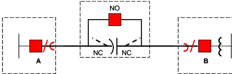
In Figure 2, the series reactor and in-line switches are part of the AC Circuit since they are within the AC Circuit boundaries even though they are within the AC Substation boundaries. In Figure 3, they are not part of the AC Circuit because they are not within the AC Circuit boundaries.
