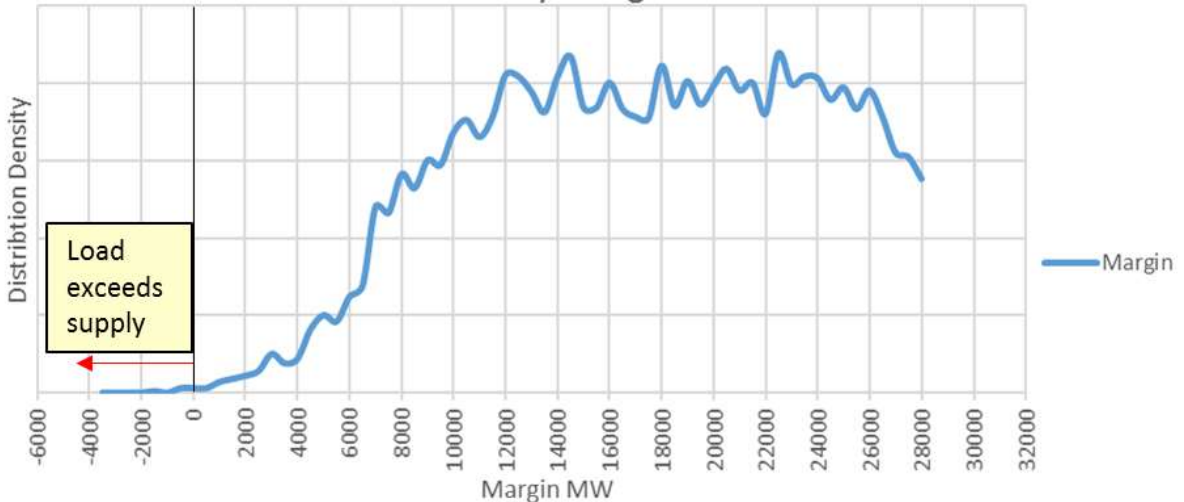
Figure 2.6: Conceptual Margin Between Loads and Mix with Wind, Solar, and Fewer Dispatchable Resources
