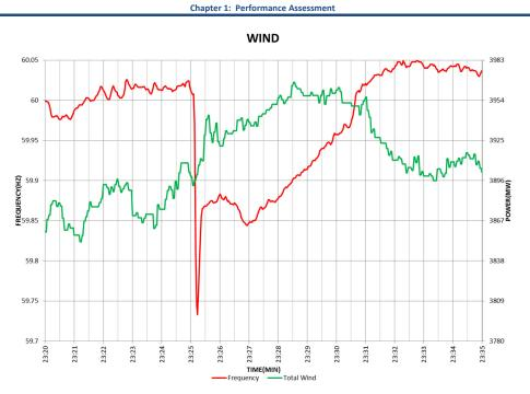
Figure A.4: Wind Resources Responding to Low Frequency Event at 17 mHz Deadband and Five Percent Droop
