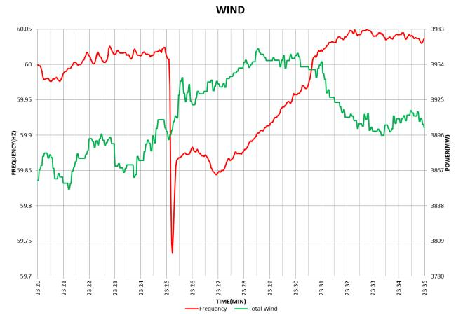
Figure A.4: Wind Resources Responding to Low Frequency Event at 17 mHz Deadband and Five Percent Droop
