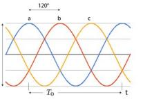
$T_{\rm O}$  = one rotor revolution if single pole pair
