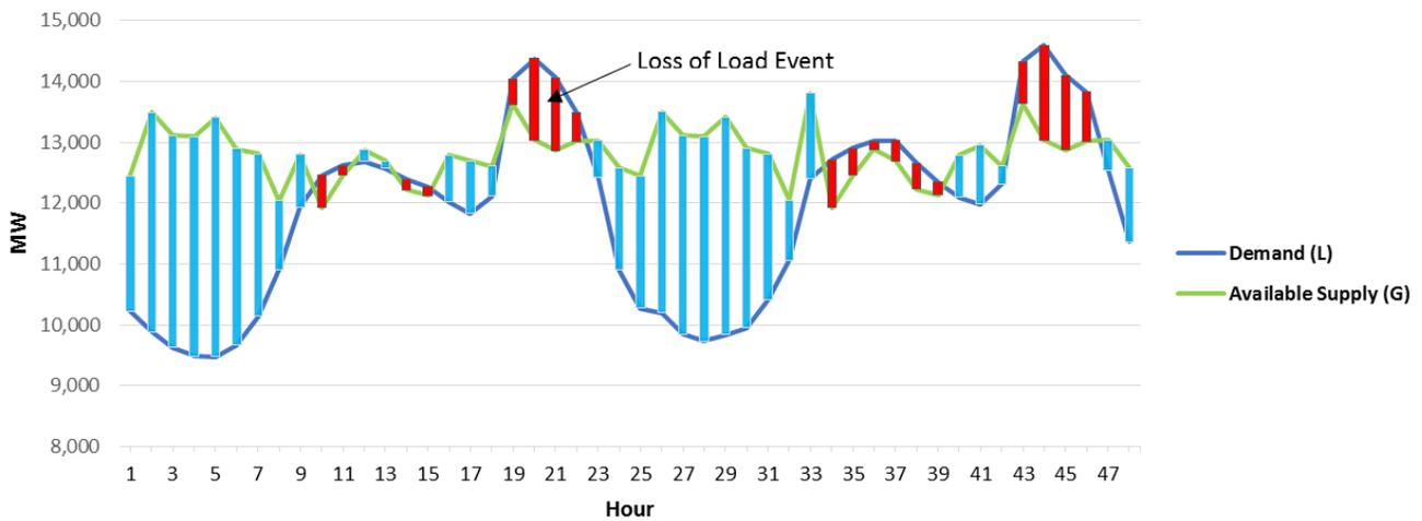
Figure C.1: Generic System Loss of Load Events—Iteration 2
