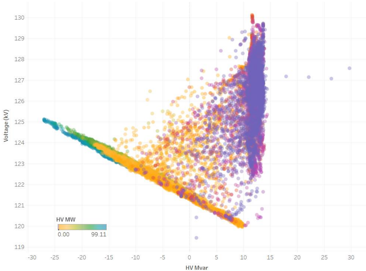
Figure 1.3: 100 MW Wind Farm Droop Characteristic and Active Power Output [Source: IESO]
