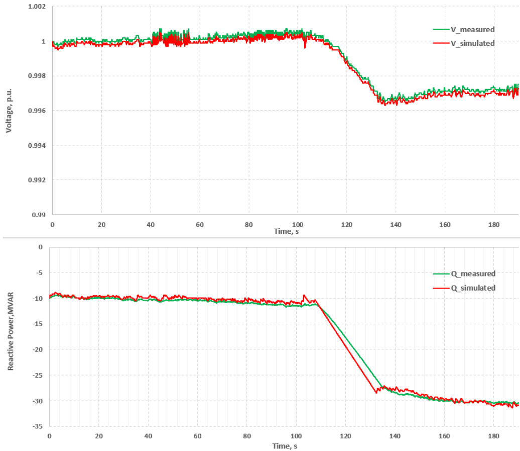
Figure 4.6: Voltage Reference Step Test at Solar PV Plant with No Local Inverter Voltage Controls (Plant-Level Control Only)
