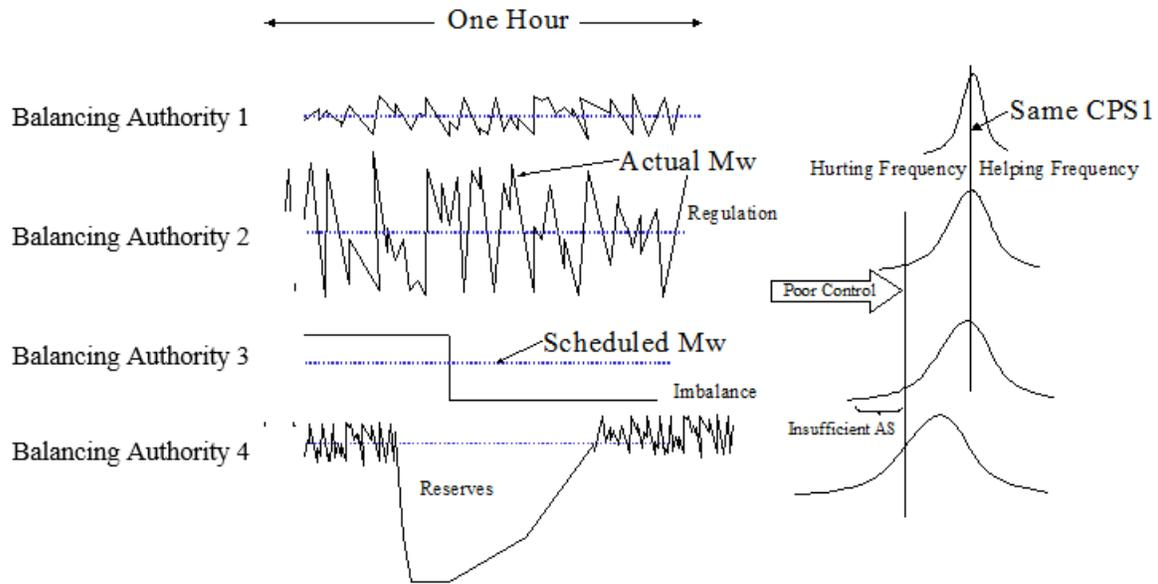
**Figure 3.3: ERS/Ancillary Service Measured via CPS1**
