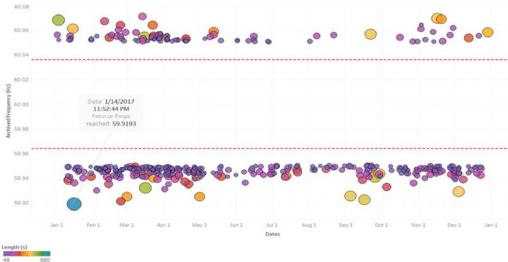
Figure 2.2: Illustration of Frequency Excursions in 2017 in the Eastern Interconnection [Source: IESO]
