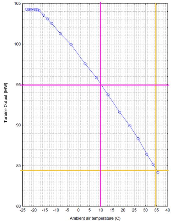
**Figure 1.13: Capability and Ambient Temperature Curves [Source: IESO]**
