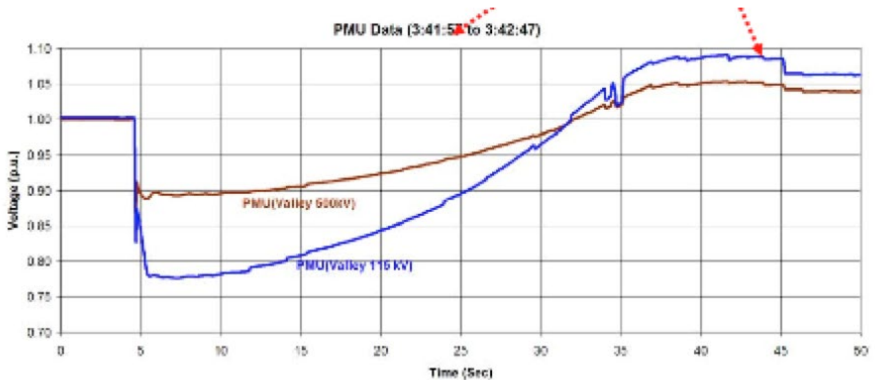
Figure 2.2: 500 and 115 kV Bus Voltage for a Three-Phase Fault Cleared in Two Cycles
