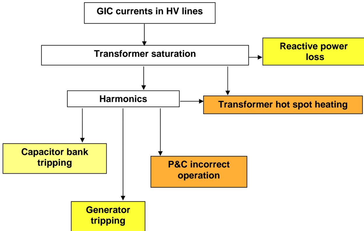
**Fig. 4:** Effects of GIC on the power system
