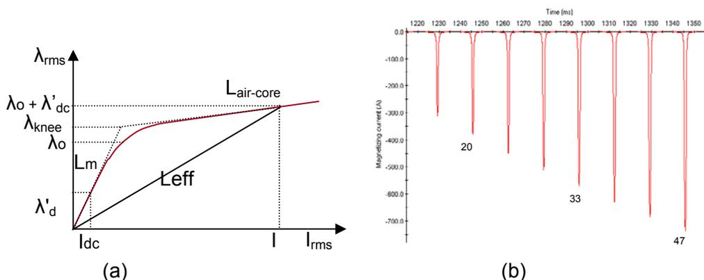
**Fig. 3:** (a) RMS flux vs. RMS current. (b) Magnetizing currents for increasing values of dc flux bias.
