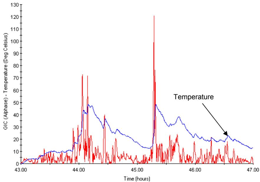
**Fig. 11:** Incremental temperature rise of the tie plate of a single-phase 500/16.5 kV 400 MVA transformer under a pre-recorded GMD event. Blue trace is the estimated temperature and the red trace is the absolute value of the GIC in the winding.
