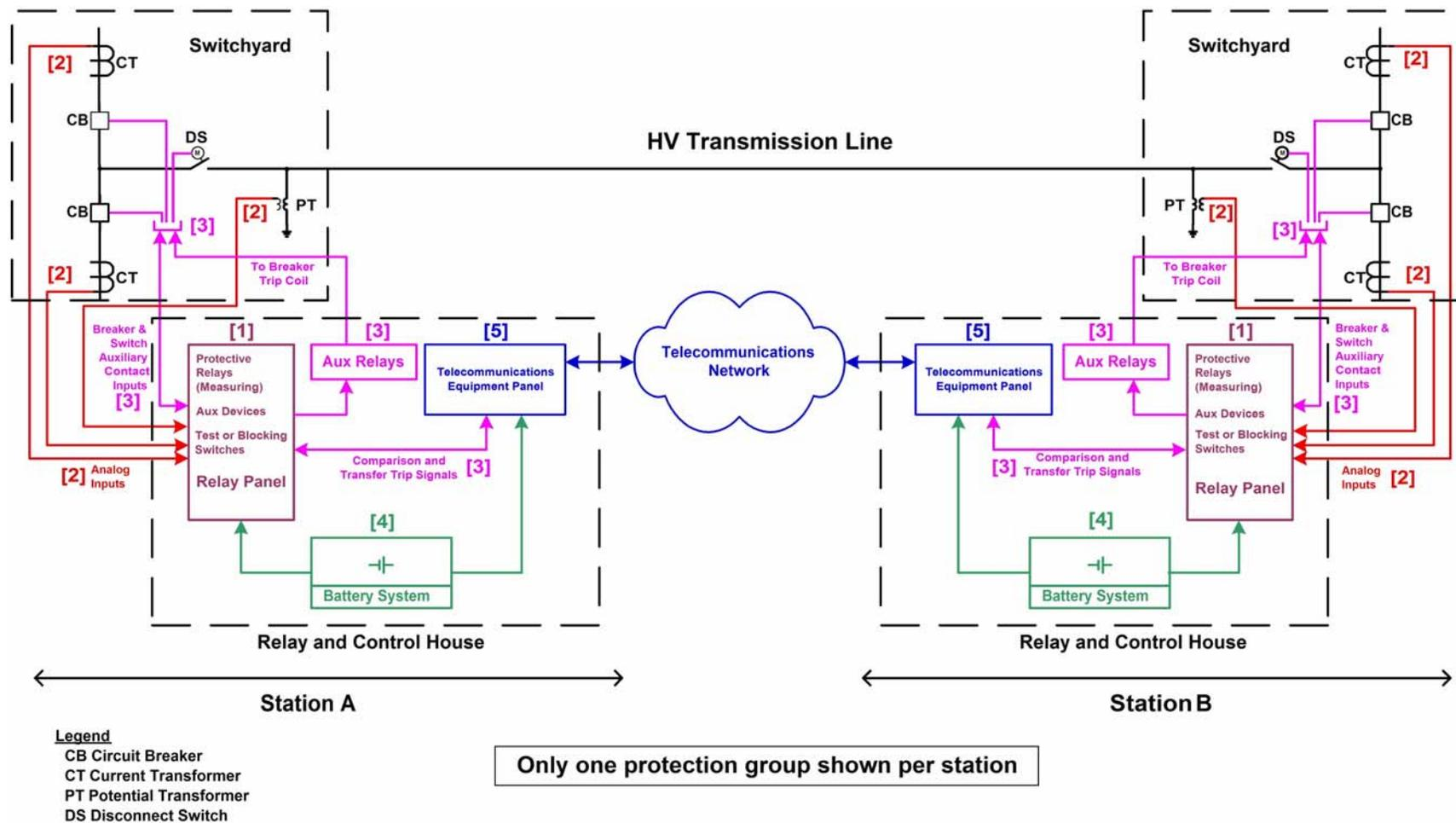
Figure 1 – Transmission Line Protection System with Identification of Equipment Categories
