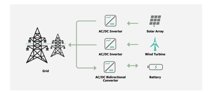
NERC uses the term "inverter-based resource" to refer generally to BPS-connected facilities that have a power electronic interface between the ac grid and the source of electricity.
