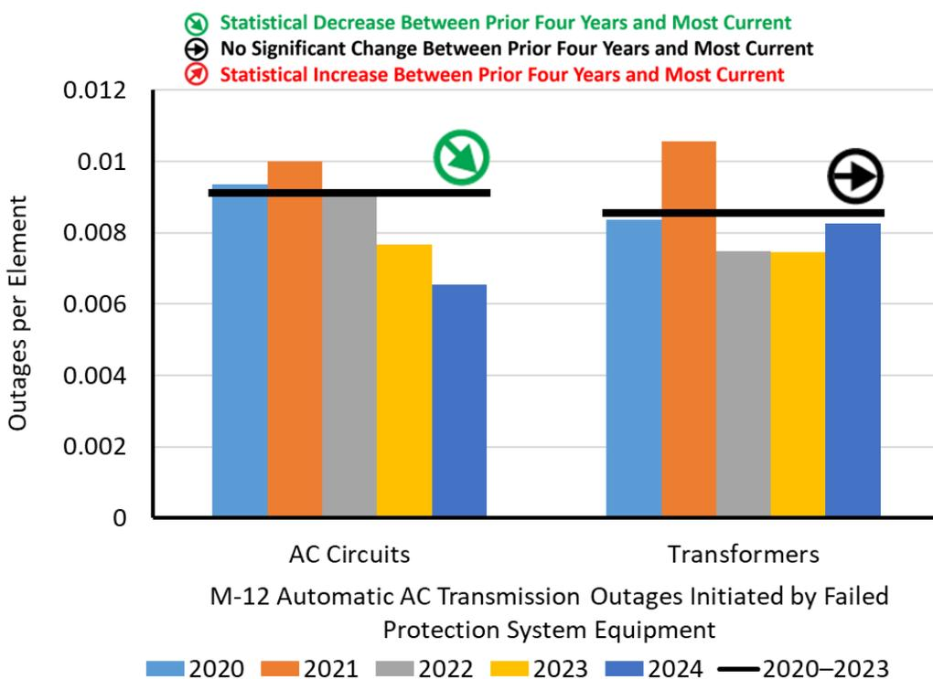
**Figure 3.8: Failed Protection System Equipment Outages<sup>55</sup>**
