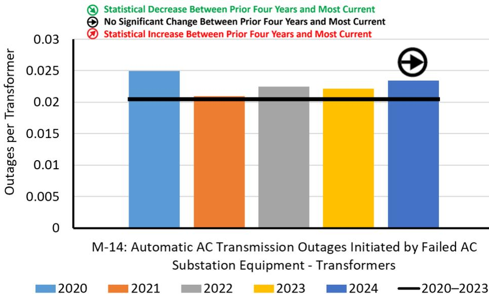
**Figure 4.18: Number of Outages Per Transformer Due to Failed AC Substation Equipment<sup>80</sup>**
