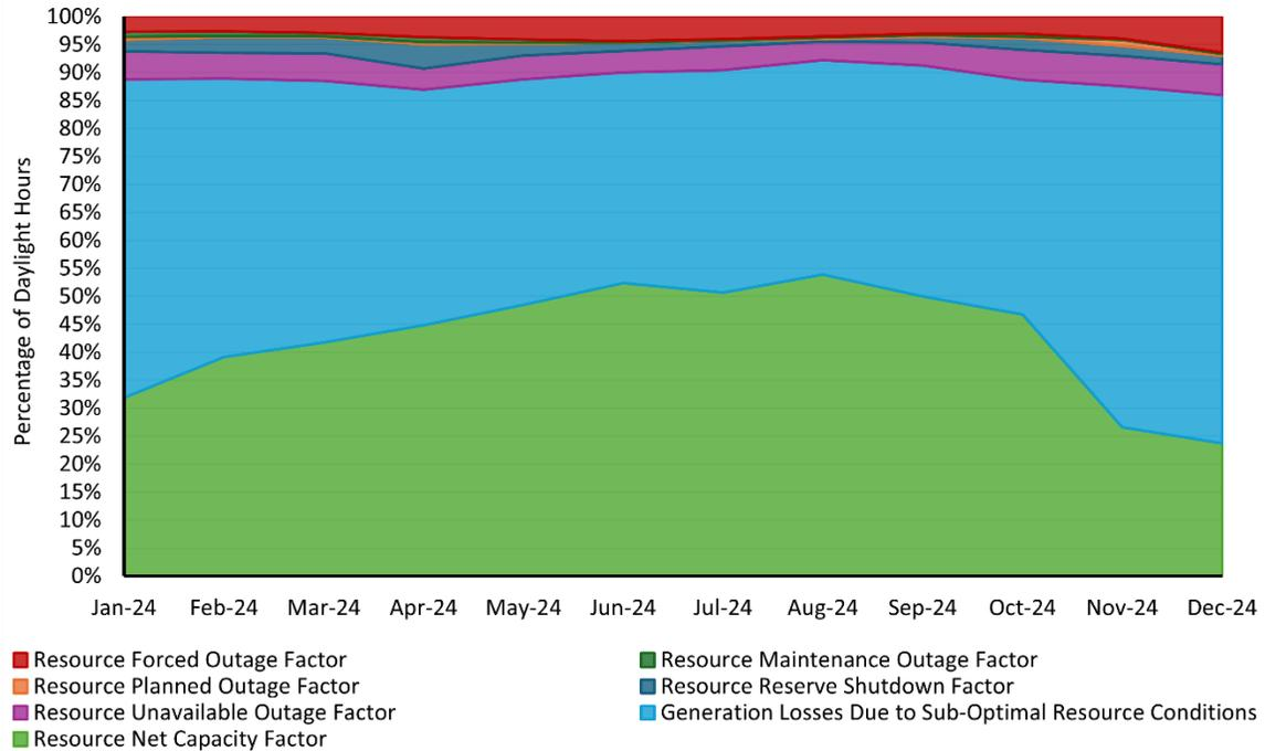
**Figure 4.11: Monthly Factors for Solar Plants >100 MW, Daylight Hours**
