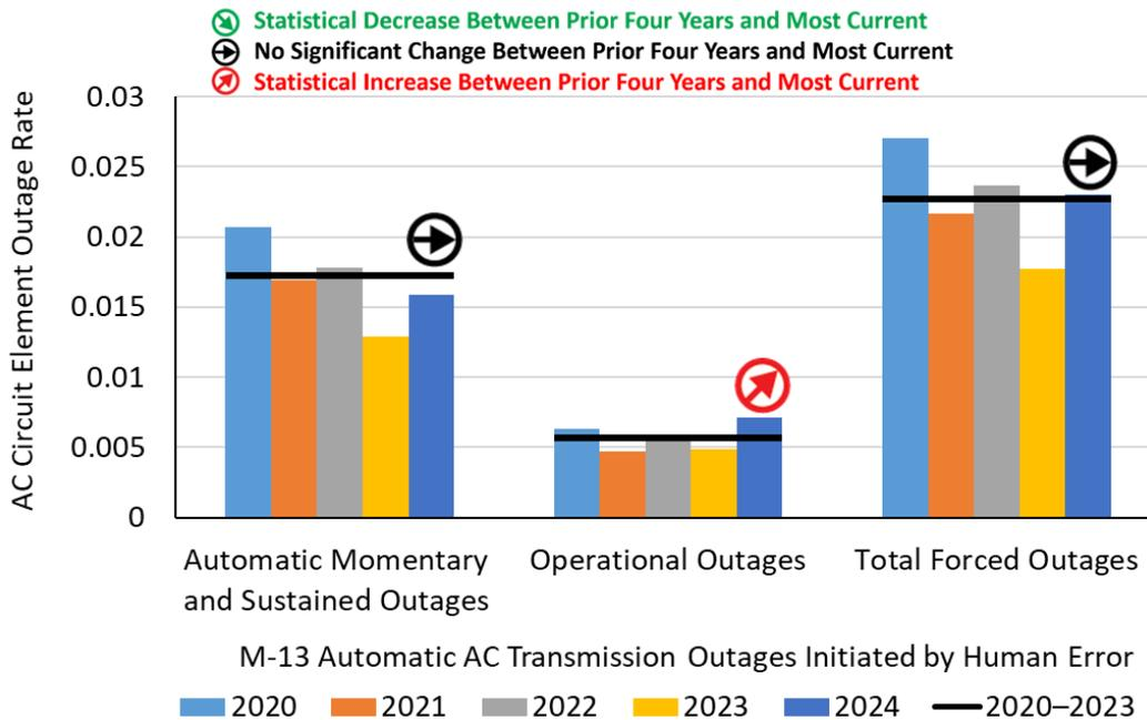
**Figure 3.14: AC Circuit Outages Per Circuit Initiated by Human Error<sup>65</sup>**
