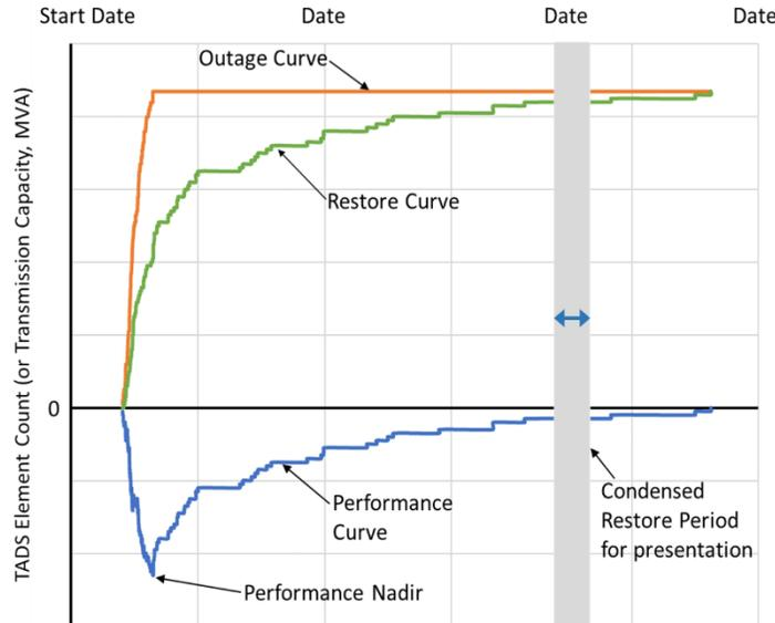
**Figure 2.5: Example of Outage, Restore, and Performance Curves for a Large Transmission Outage Event**
