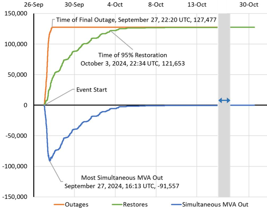
**Figure 2.8: Transmission Capacity (MVA-Based) Outage, Restore, and Performance Curve for Hurricane Helene, September 27–October 30, 2024**
