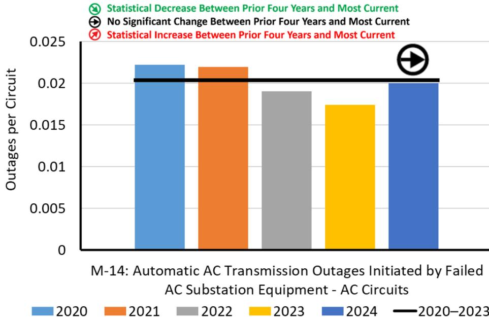
**Figure 4.16: Number of Outages Per AC Circuit Due to Failed AC Substation Equipment<sup>78</sup>**
