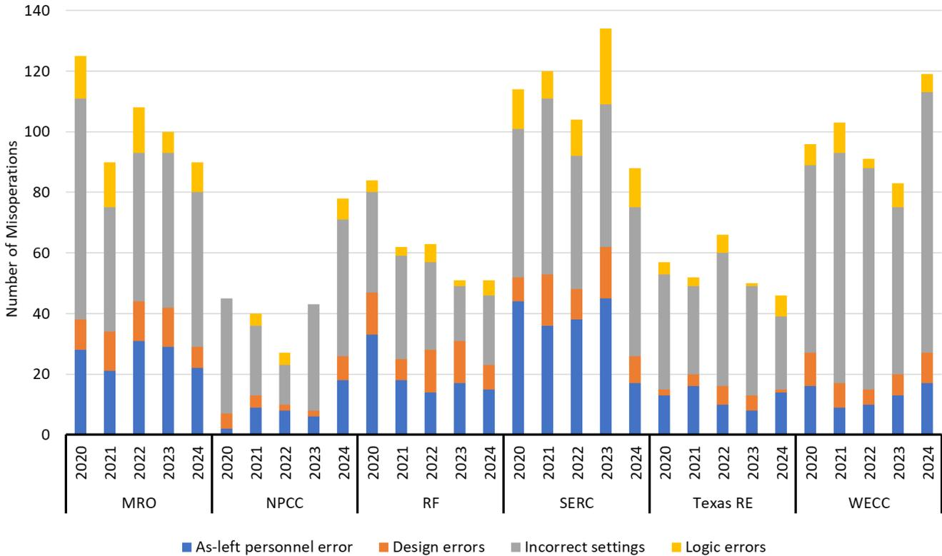
**Figure 3.17: MIDAS Protection System Misoperations Due to Human Error by Regional Entity**
