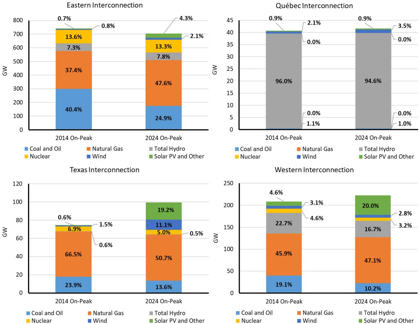
**Figure 3.4: 2014 and 2024 Capacity Resource Mix by Interconnection**
