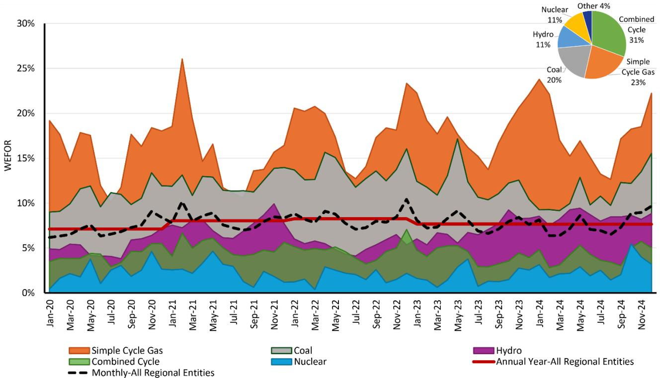
**Figure 4.6: Five-Year WEFOR by Fuel Type and 2024 Resource Mix by Net Maximum Capacity**
