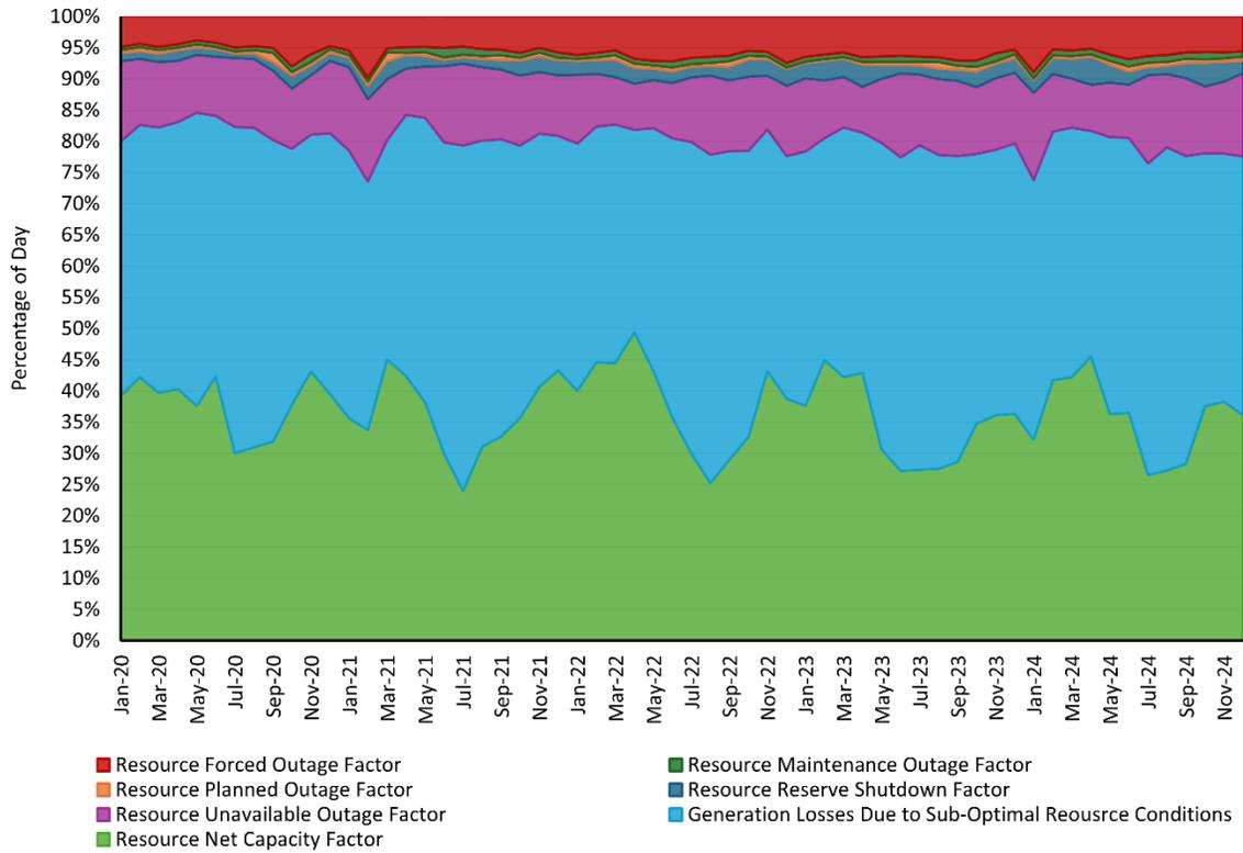
**Figure 4.8: Monthly Net Output Factor and Weighted Resource Forced Outage Rate (WRFOR) Wind Plant Reporting Group 200 MW+**
