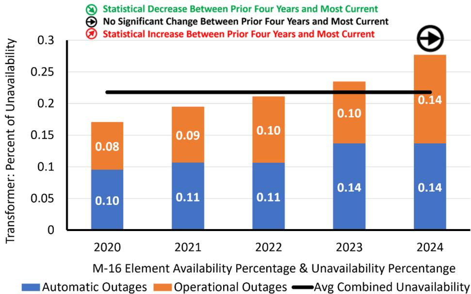
**Figure 4.20: Transformer Unavailability >200 kV<sup>82</sup>**
