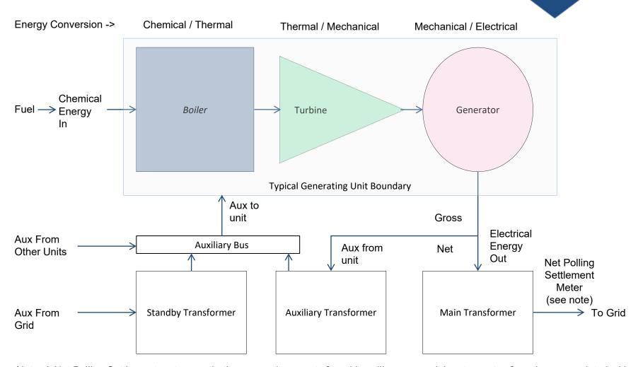
Note: A Net Polling Settlement meter runs both ways and accounts for grid auxiliary power; it has two sets of numbers associated with it: 1) Adjusted for grid auxiliary power, and 2) Unadjusted which just shows the power out of the high side of the main transformer.
