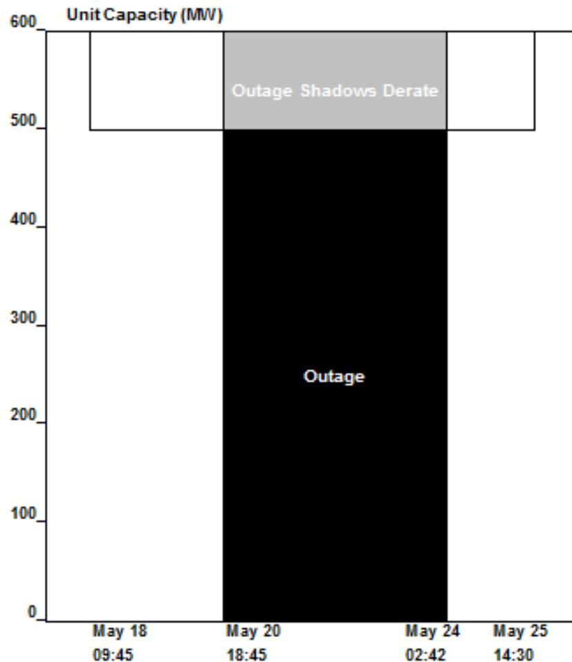
Figure G-6B — Derate Overlapped by an Outage
