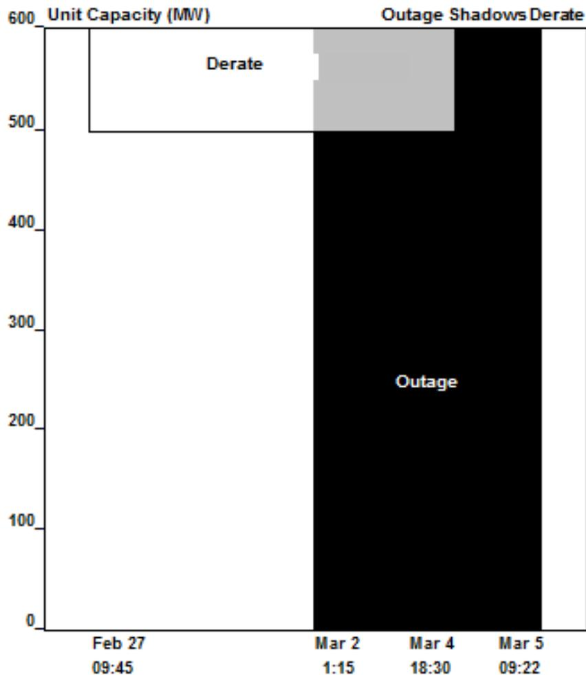
Figure G-6A— Derate Overlapped by an Outage
