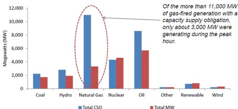
**Figure 3: ISO-NE Generator Capacity Supply Obligations vs. Output (January 28, 2014)**
