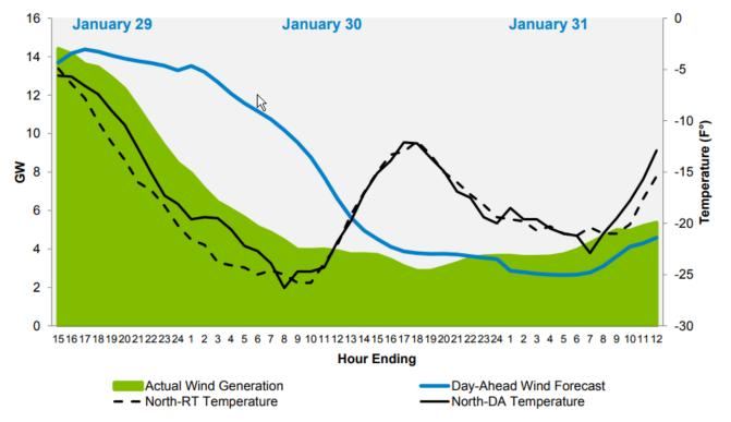
Figure 5: MISO Wind Generation during January 2019 Cold Snap [Source: MISO]
