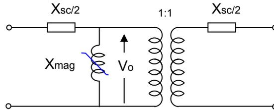
**Fig. 1:** Simplified representation of a single-phase transformer
