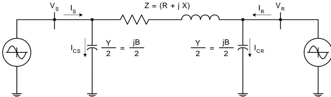
Lengthy transmission lines have significant series resistance, reactance, and shunt capacitance. The line resistance consumes real power when current flows through the line and increases the real power input during maximum power transfer. The shunt capacitance supplies reactive current, which impacts the sending end reactive power requirements of the transmission line during maximum power transfer. These line parameters should be used when calculating the maximum line power flow.
