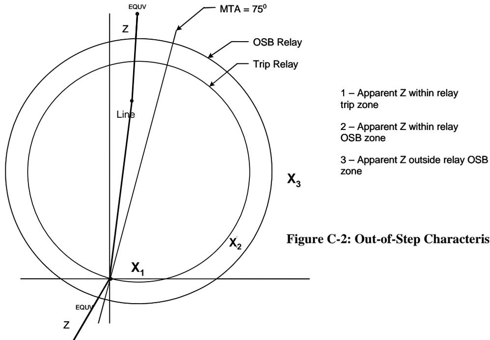
**Figure C-2: Out-of-Step Characteristics with Load**
