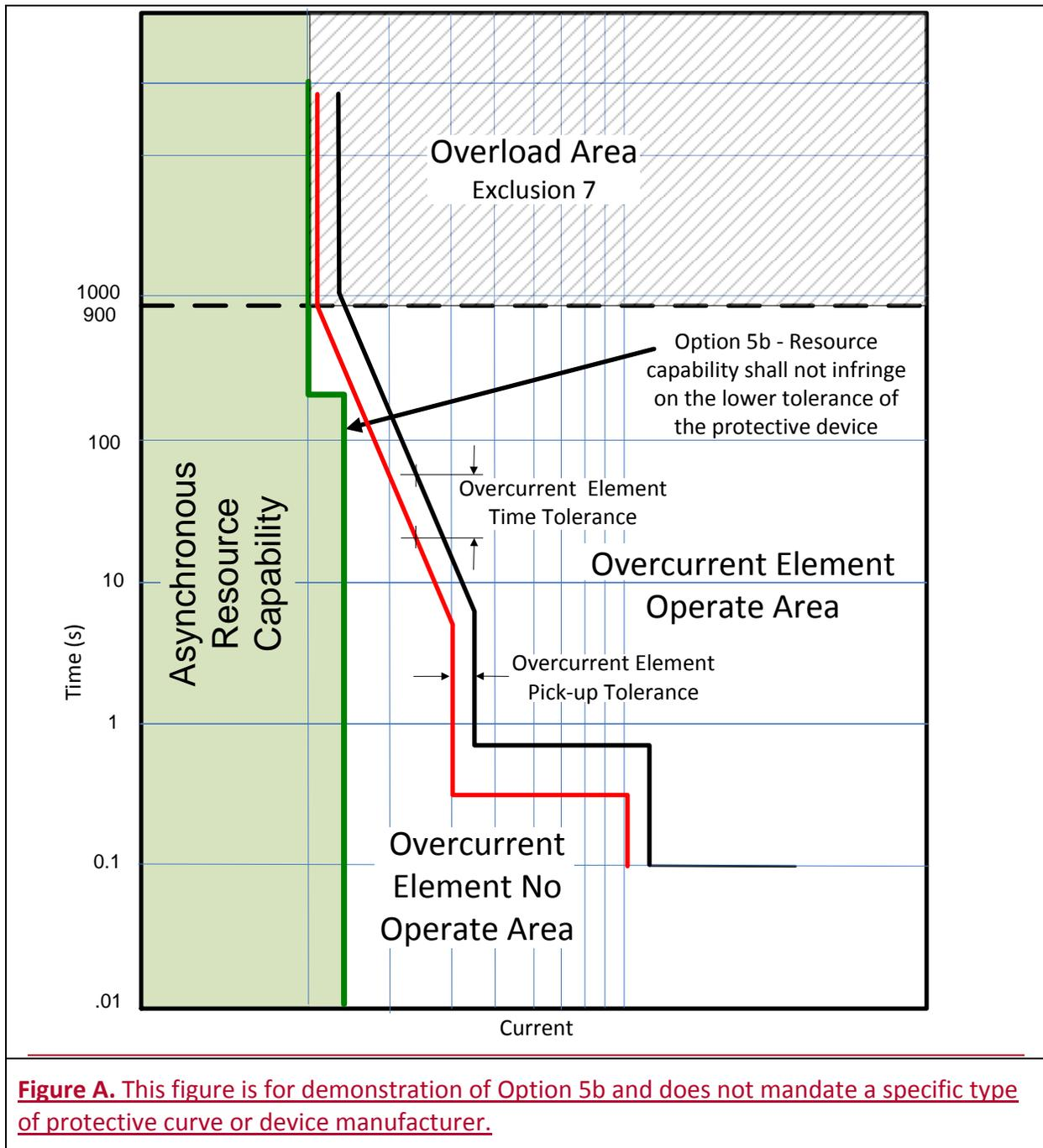
**Figure A.** This figure is for demonstration of Option 5b and does not mandate a specific type of protective curve or device manufacturer.
