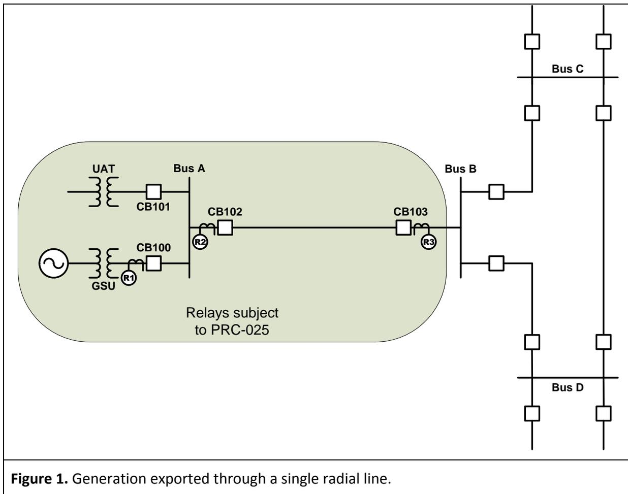
**Figure 1.** Generation exported through a single radial line.
