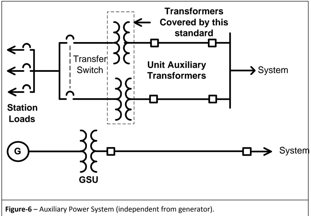
Figure-6 – Auxiliary Power System (independent from generator).
