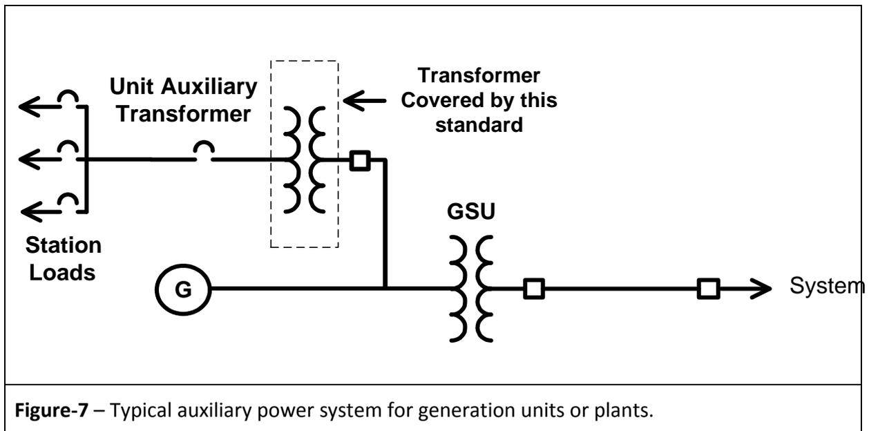
The UATs supplying power to the unit or plant electrical auxiliaries are sized to accommodate the maximum expected overall UAT load demand at the highest generator output. Although the transformer nameplate MVA size normally includes capacity for future loads as well as capacity for starting of large induction motors on the original unit or plant design, the nameplate MVA capacity of the transformer may be near full load.
