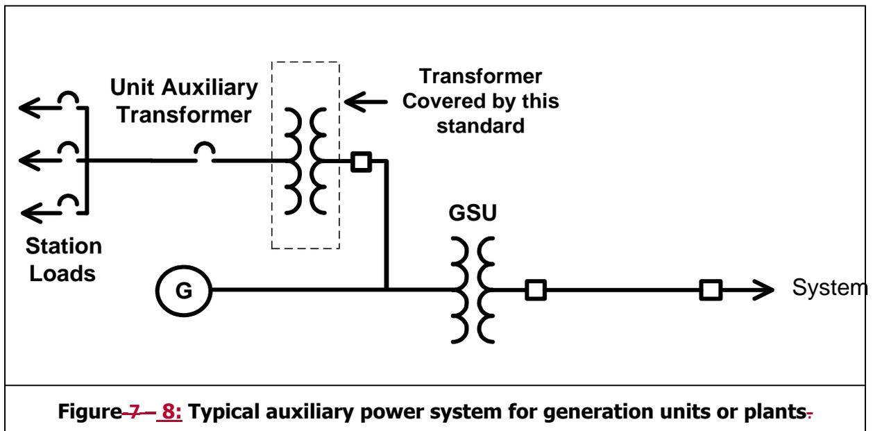
**Figure-~~7-8~~: Typical auxiliary power system for generation units or plants.**
