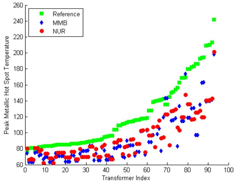
**Figure I-7: Calculated ~~peak metallic hot spot temperature~~ Peak Metallic Hot Spot Temperature for ~~all transformers~~ All Transformers in a ~~test system~~ Test System with a ~~temperature increase~~ Temperature Increase of ~~more than~~ More Than 20°C for ~~different GMD events scaled~~ Events Scaled to the ~~same peak geoelectric field~~ Same Peak Geoelectric Field**
