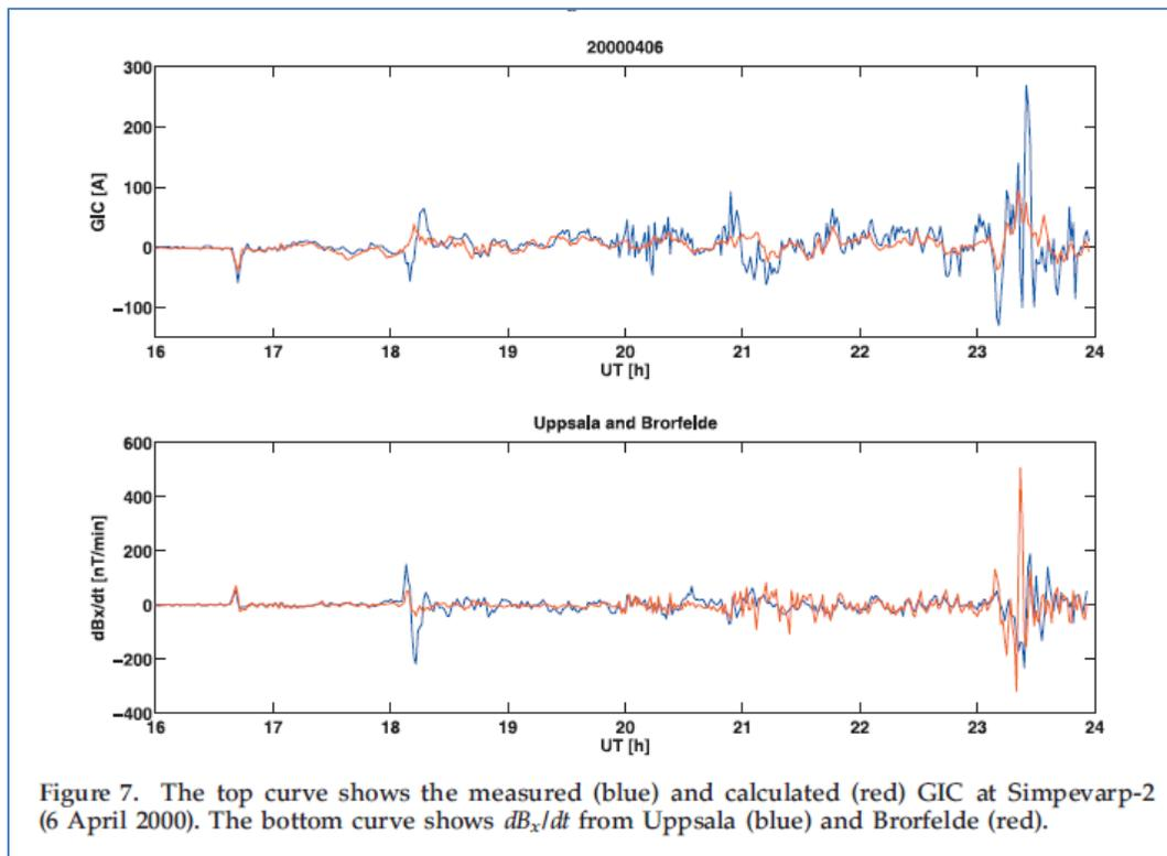
Figure 7. The top curve shows the measured (blue) and calculated (red) GIC at Simpevarp-2 (6 April 2000). The bottom curve shows  $dB_x/dt$  from Uppsala (blue) and Brorfelde (red).
