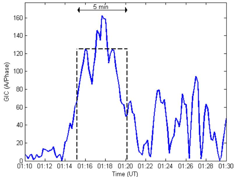
**Figure 16: Close-up of  $GIC(t)$  and a 5 minute GIC pulse assuming 70% load**
