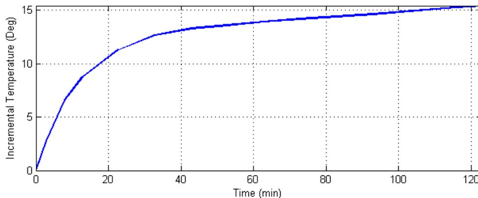
**Figure 7: Thermal Step Response to a 5 A/phase dc Step [3]
