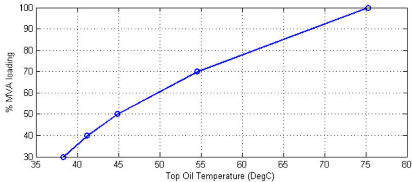
**Figure 13: Simplified loading curve assuming 30°C ambient temperature**
