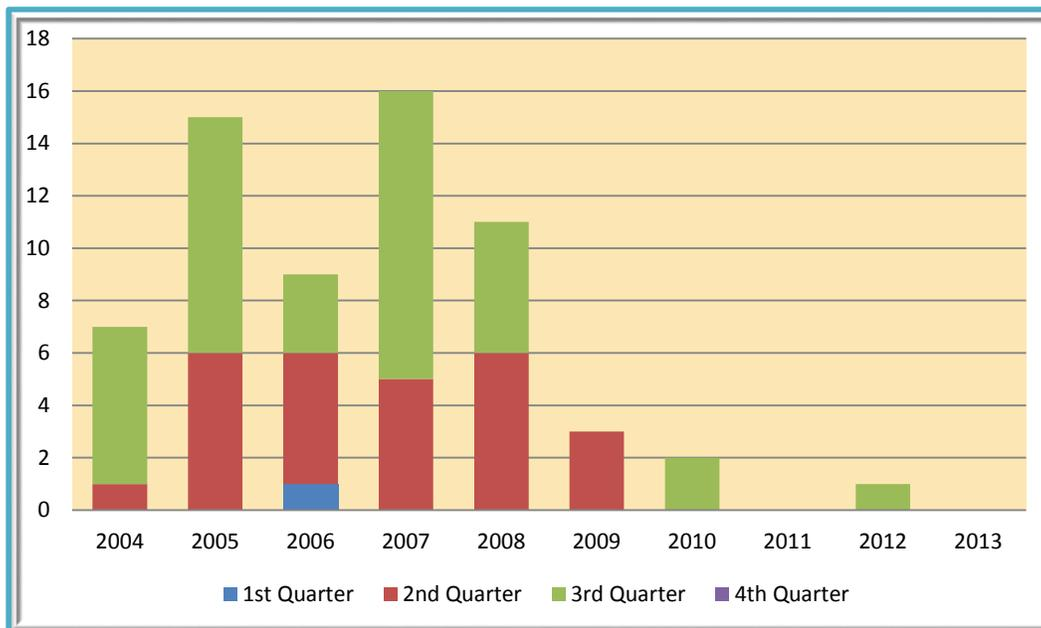
Figure 1: Category 1 — Grow-in Outages Caused by Vegetation Growing into Lines from Inside and/or Outside the ROW.<sup>5</sup>
