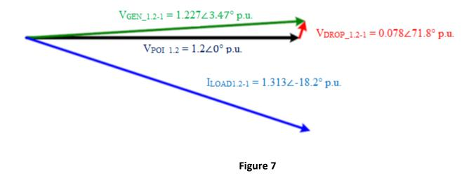
Rotate the load-flow current by the difference of power factor angle between the POI and the generator calculated in the first iteration to obtain the desired generator power factor angle for the next iteration.
