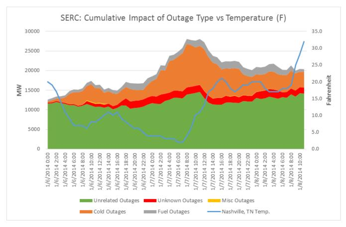
Figure 10: SERC: Cumulative Impact of Outage Type vs. Temperature (F)
