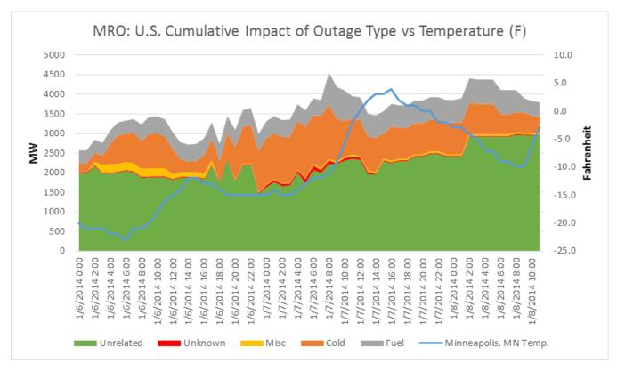
Figure 7: MRO (US): Cumulative Impact of Outage Type vs. Temperature (F)
