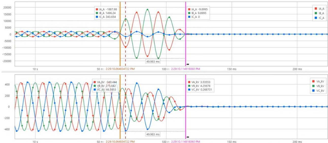
**Figure 1.6: Fault Clearing for August 25 Disturbance**
