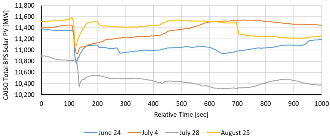
**Figure 1.2: CAISO BPS-Connected Solar PV during Disturbance**
