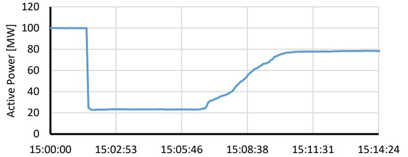
feeders that have an underground collector portion; the inverters that remained on-line are located on a fully-overhead collector system. The plant owner also stated that the voltage ride-through protection had been disabled in May 2021 unexpectedly during maintenance procedures and were restored at the end of August 2021. It is unclear if this was a contributor to this resource tripping abnormally for this event.
