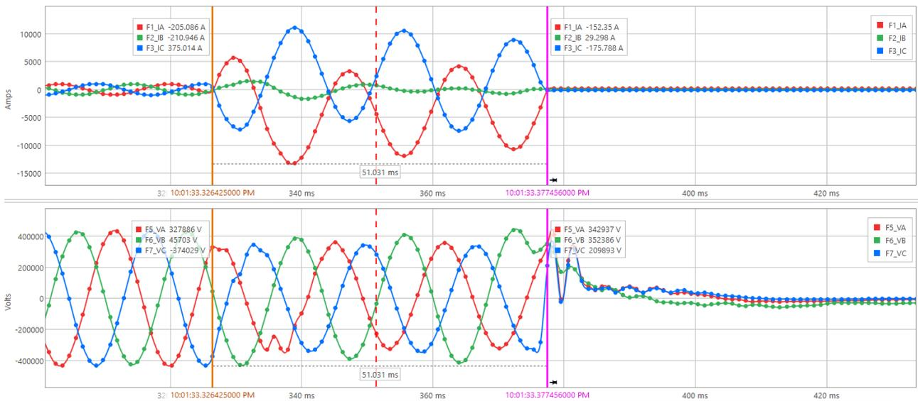
Figure 1.4: Fault Clearing for July 4 Disturbance
