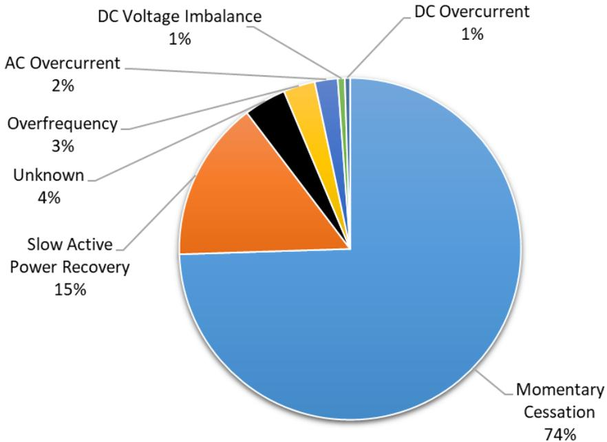
**Figure 2.4: August 25 Disturbance Causes of Solar PV Reductions**
