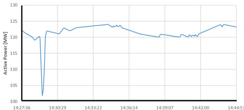
**Figure 2.6: Example of Slow Active Power Recovery Following Fault**
