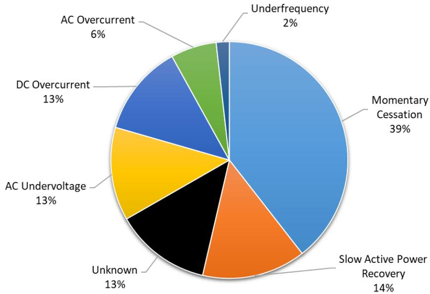
**Figure 2.1: June 24 Disturbance Causes of Solar PV Reduction**
