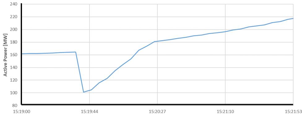
**Figure 2.5: Example of Plant Prolonged Active Power Recovery Post-Fault**
