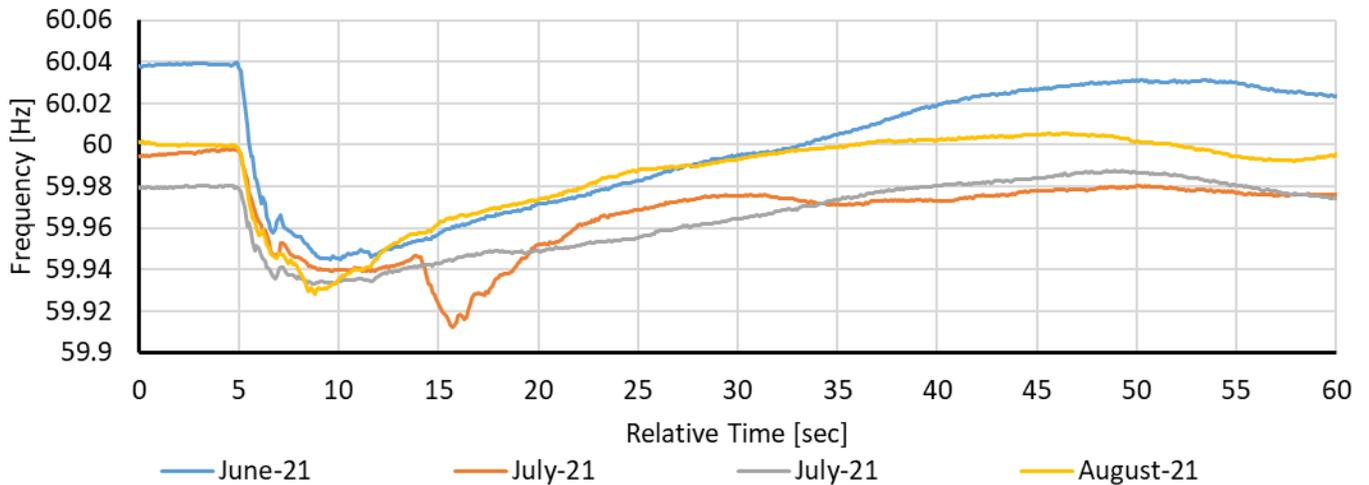
**Figure 1.11: System Frequency Response for Each Disturbance [Source: UTK/ORNL]**
