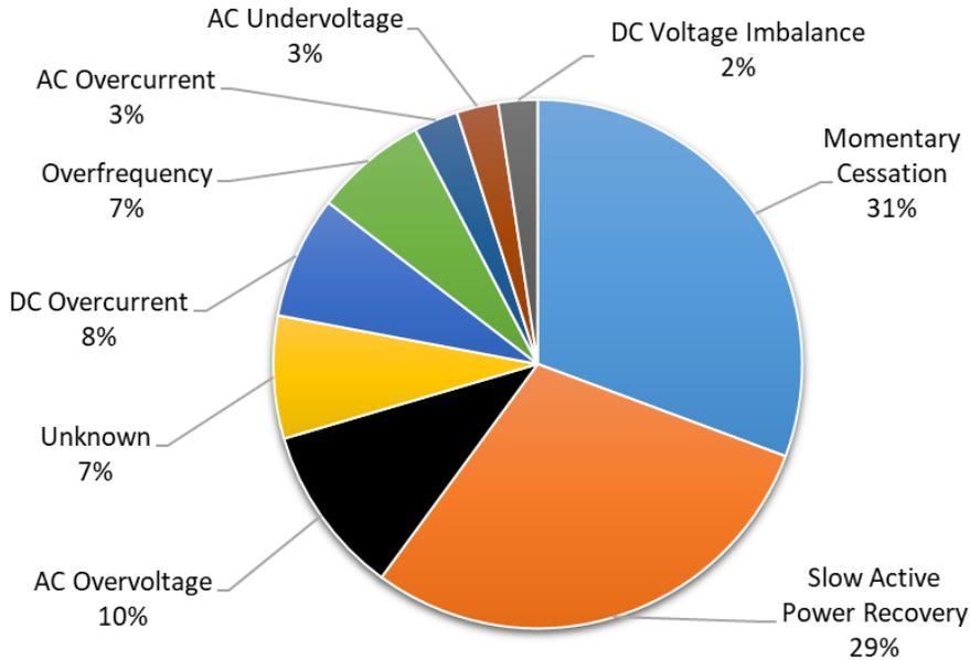
**Figure 2.3: July 28 Disturbance Causes of Solar PV Reduction**
