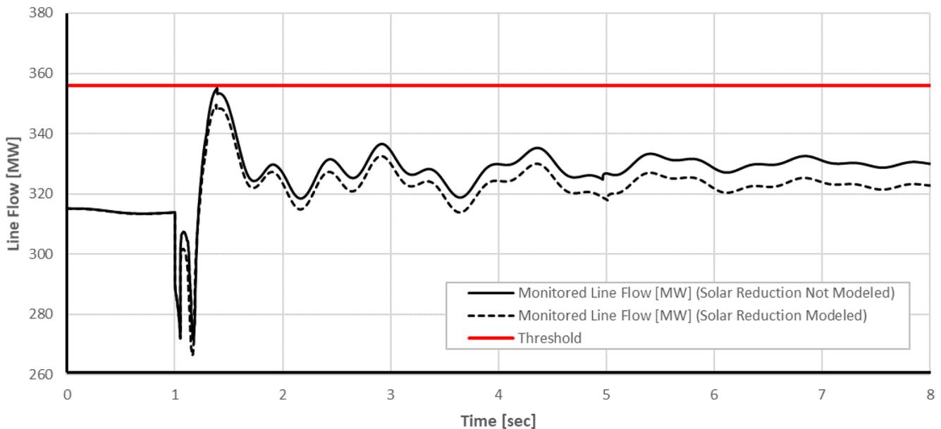
**Figure C.1: Simulation of RAS Operation with and without Solar PV Modeled**
