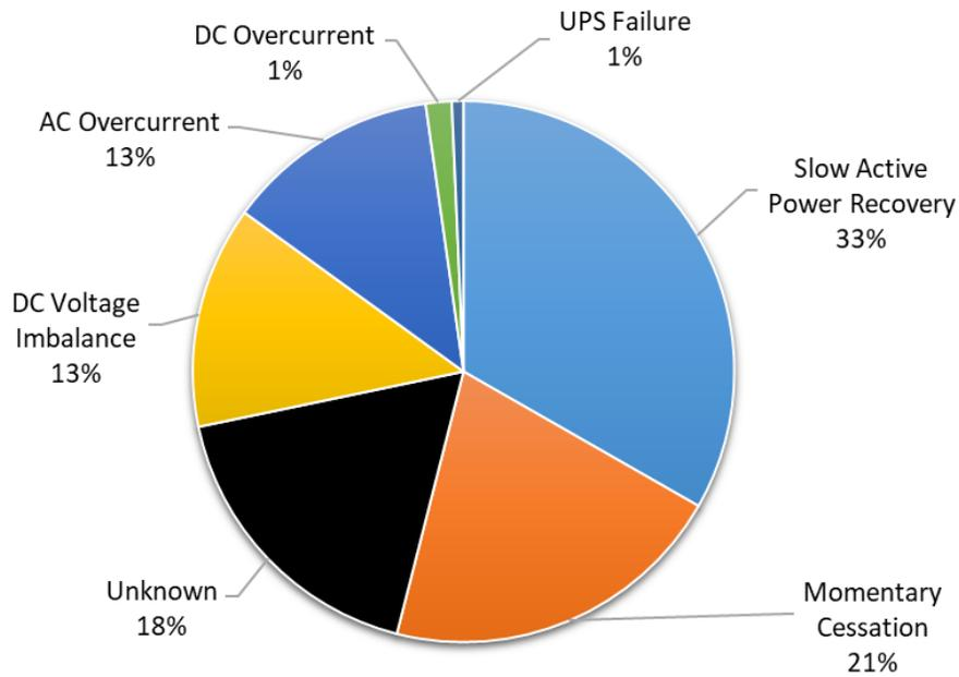
**Figure 2.2: July 4 Disturbance Causes of Solar PV Reduction**
