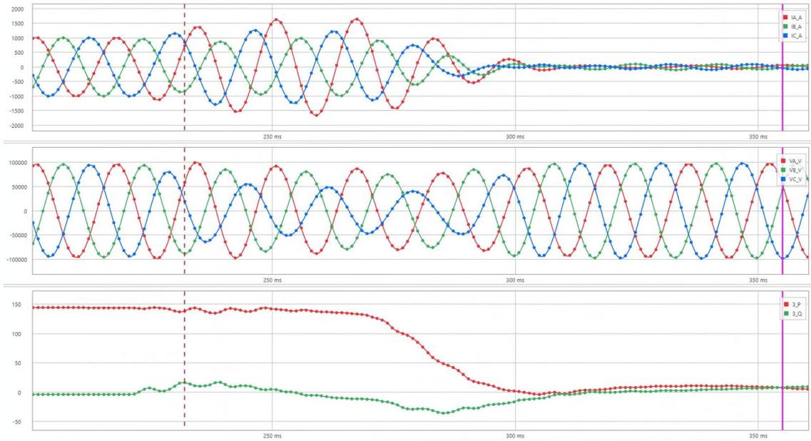
**Figure B.2: High Speed Oscillography Data at POI Showing Plant Response to Fault**
