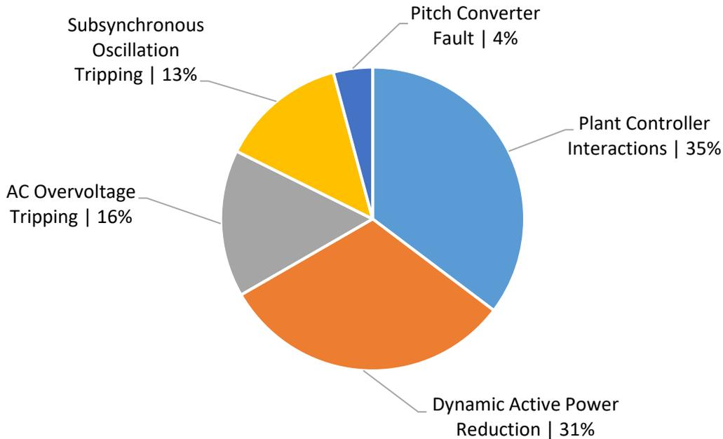
**Figure 1.2: Causes of Wind Plant Reduction for Fault 2**
