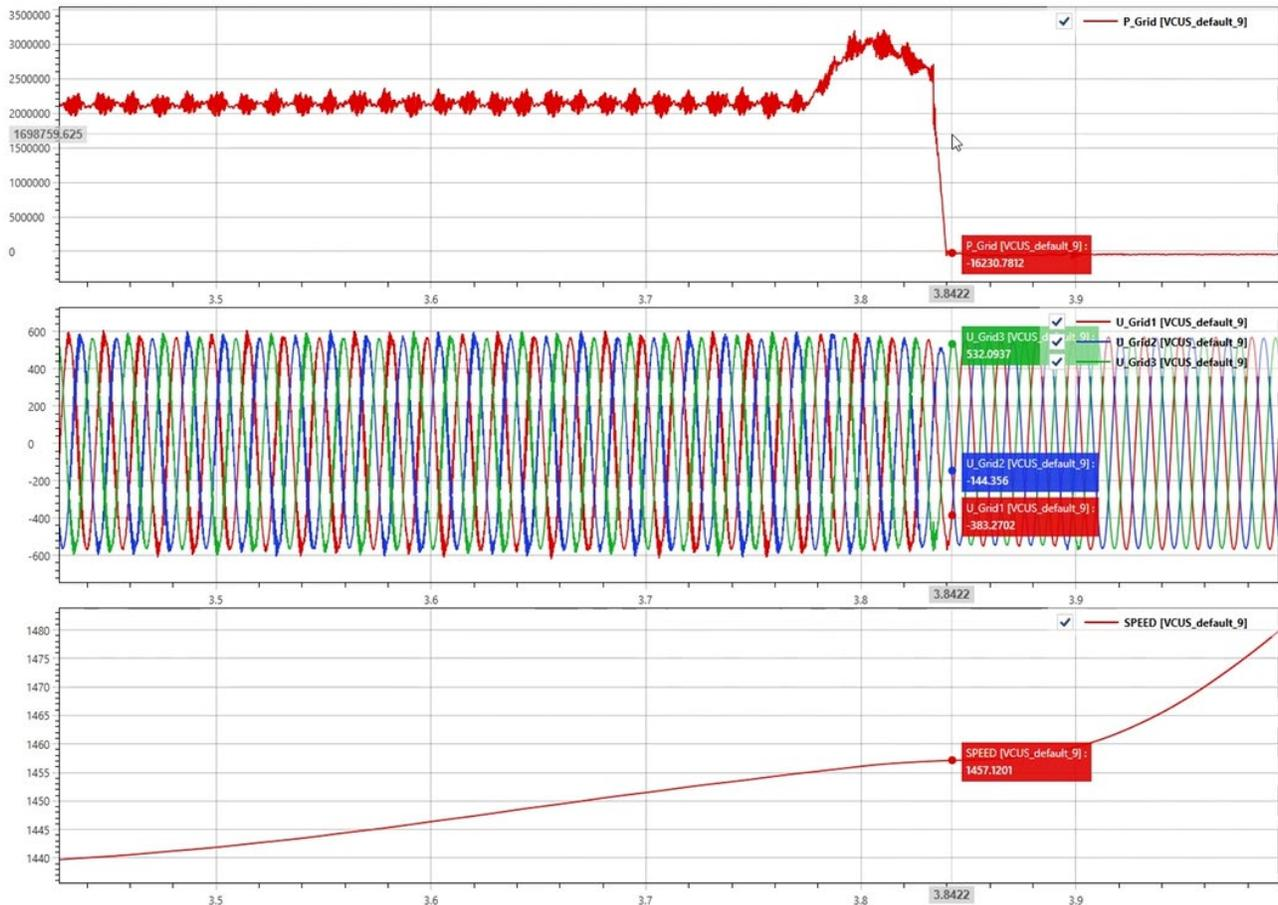
Figure 1.9: Turbine High Speed Data Capturing Turbine Tripping for Different Event
