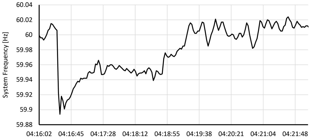
**Figure I.6: System Frequency Response for First Fault Event**
