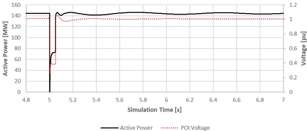
**Figure B.3: High Speed Oscillography Data at POI Showing Plant Response to Fault**
