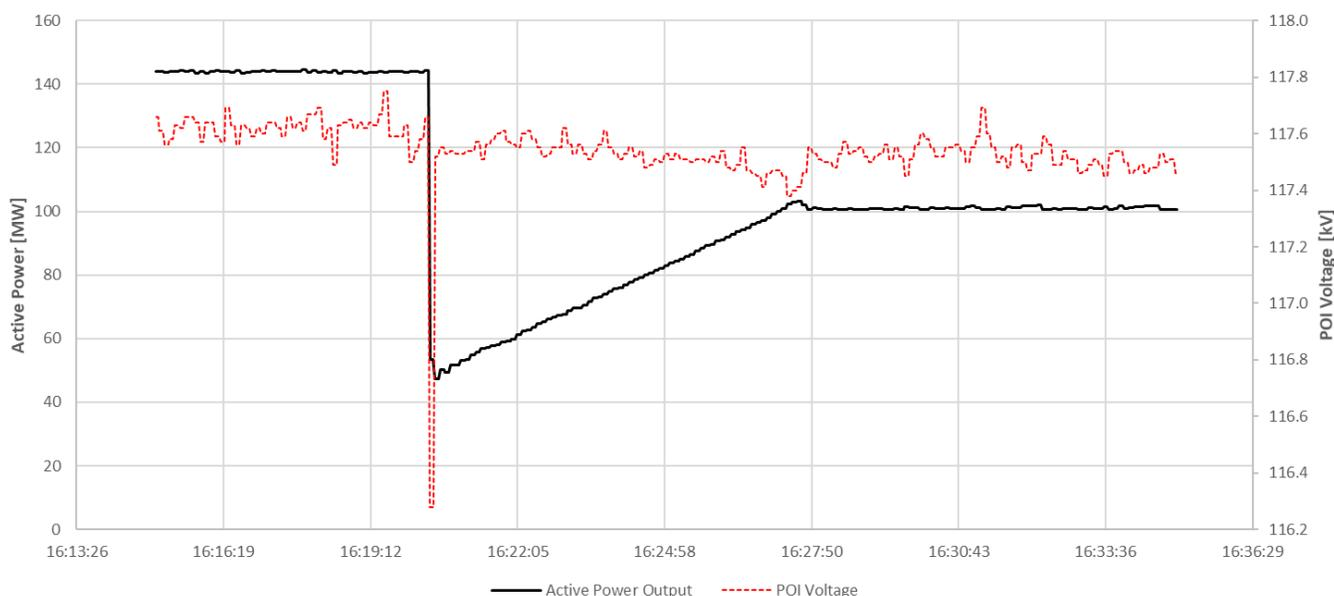
**Figure B.1: Overall Wind Plant Response to BPS Fault**
