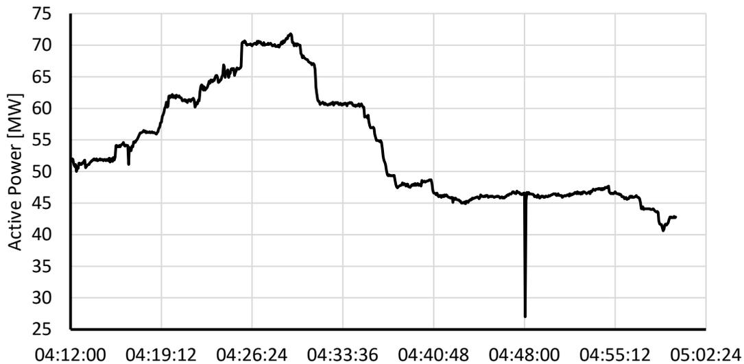
**Figure 1.4: Reduction of Active Power during Fault Conditions**
