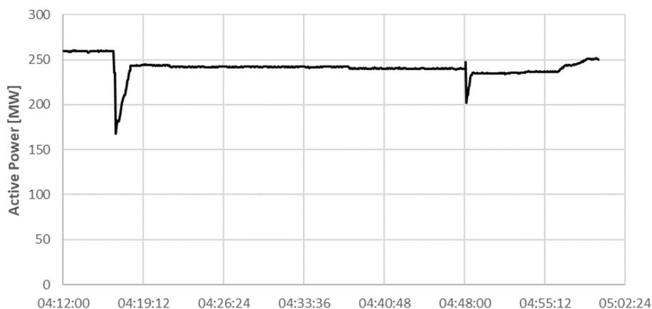
**Figure A.6: Plant Active Power Output**
