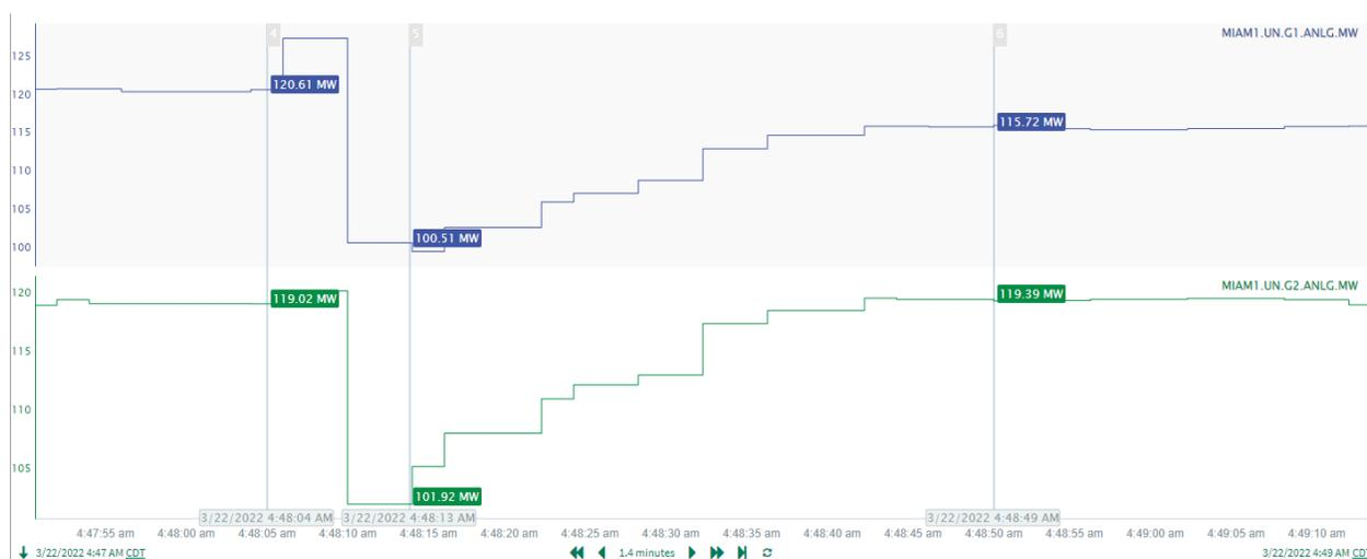
**Figure A.5: Unit 1 and Unit 2 Active Power Response to Fault 2**
