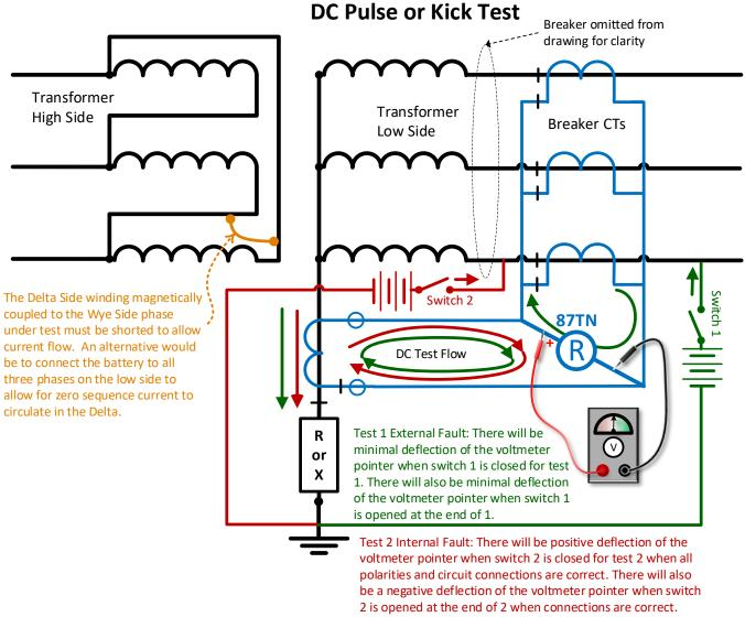
Note: Repeat the tests for all three phases.
