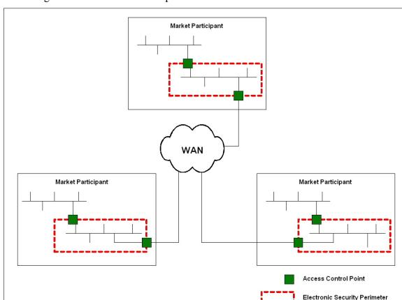
communication lines, the communication lines are not included in the Electronic Security Perimeter. The following schematic illustrates this point.
