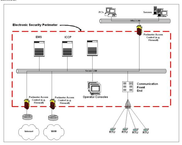
The RTUs may need an Electronic Security Perimeter if they use a routable protocol and meet the definition of a Critical Cyber Asset. Also a single computer may need an Electronic Security Perimeter if it meets the definition of a Critical Cyber Asset.
