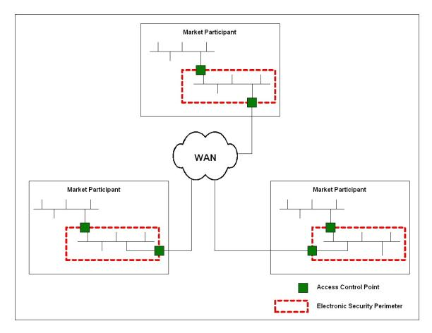
3. **Question:** I have a single RTU, which controls a critical bulk electric asset in a substation, connected through a modem to my EMS communication front-end. What is the electronic security perimeter in this case? There is no LAN in the substation.
