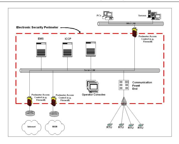
The RTUs may need an electronic security perimeter if they use a routable protocol and meet the definition of a Critical Cyber Asset. Also a single computer may need an electronic security perimeter if it meets the definition of a Critical Cyber Asset.
