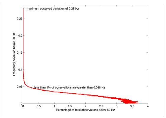
Figure 6: Texas Interconnection Frequency Deviations Below 60 Hz
