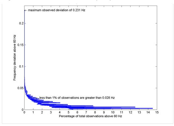
Figure 7: Québec Interconnection Frequency Deviations Above 60 Hz
