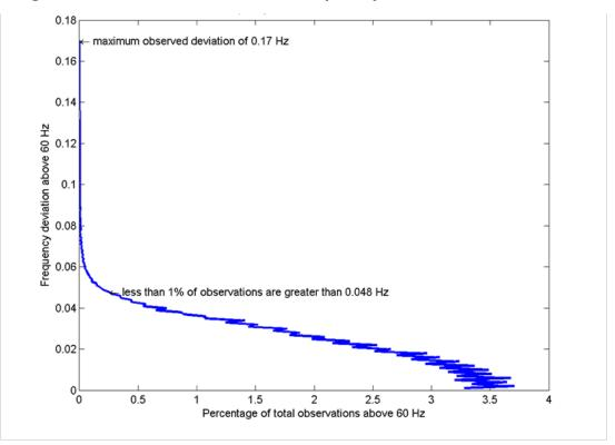
Figure 5: Texas Interconnection Frequency Deviations Above 60 Hz
