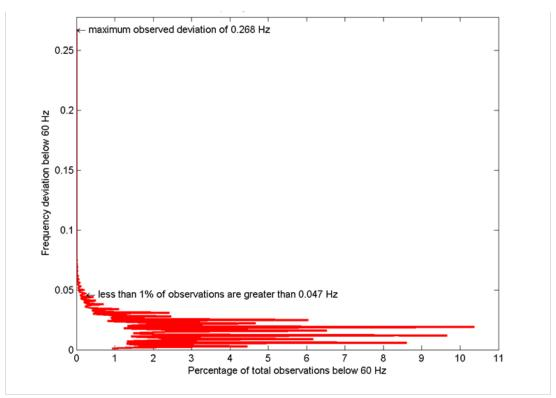
Figure 8: Québec Interconnection Frequency Deviations Below 60 Hz
