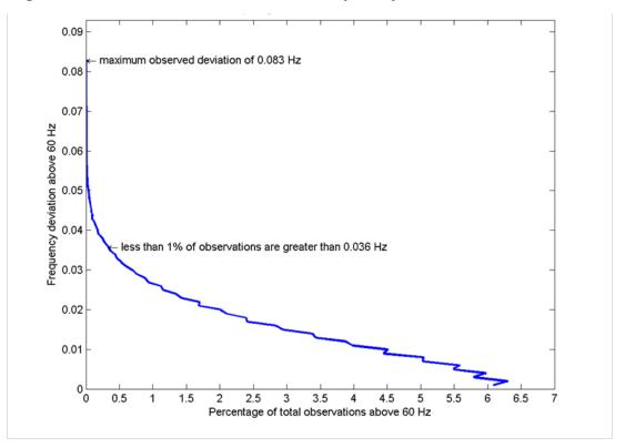
Figure 3: Western Interconnection Frequency Deviations Above 60 Hz
