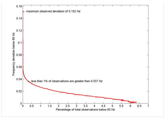
Figure 4: Western Interconnection Frequency Deviations Below 60 Hz
