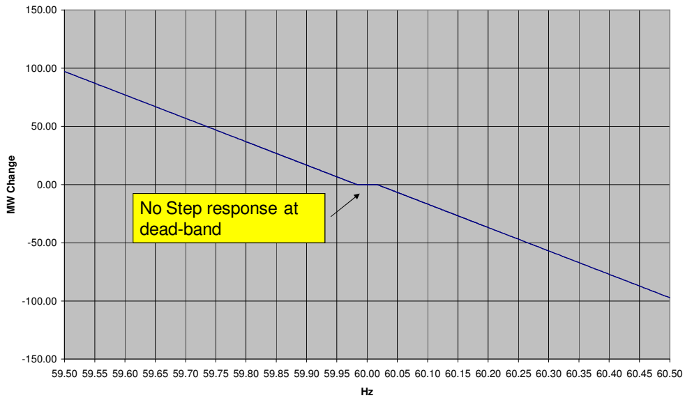
Figure T2B – Frequency Response of 600 MW Unit ±16.67 mHz Deadband and No Step Response
