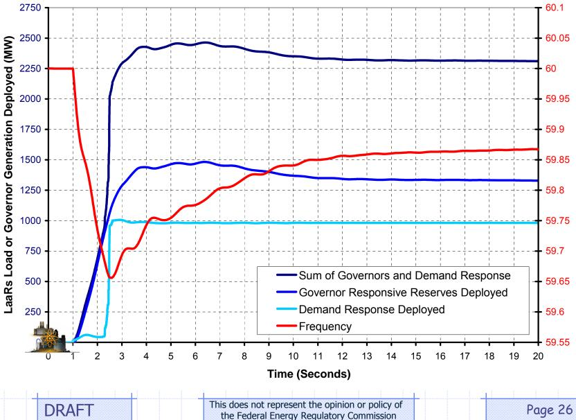
Frequency of the Eastern Interconnection following the Loss of 4,500 MW of Generation–Comparison of Recorded Data with Results from a Simulation of the Event
