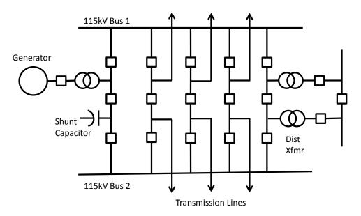
Figure 1-5 – Bus Configuration for Table B Example
