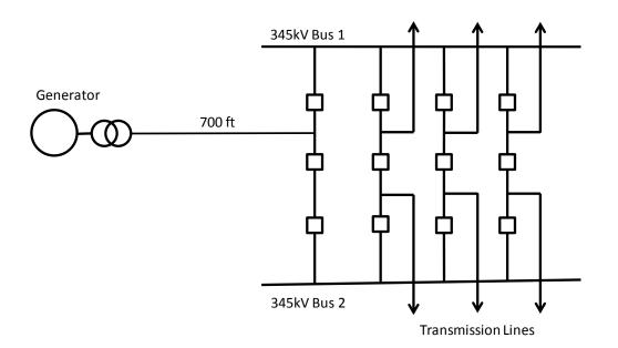
Figure 1-9 – Detailed View of Generator Connection
