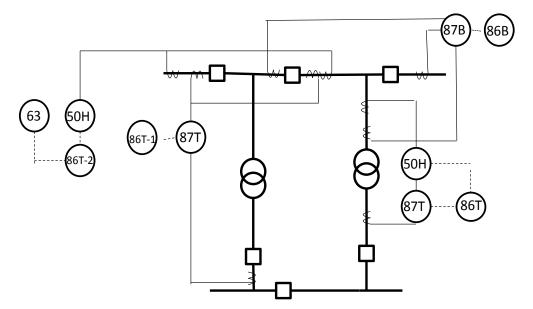
Figure 1-8 – Step-down Distribution Transformer Example
