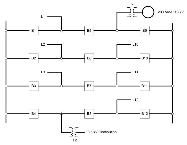
Figure 1-4 - Table A Example with a Breaker-and-a-Half Bus
