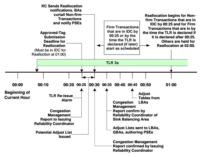
Figure 2 — Reallocation Timing for TLR 3a Called at 00:08
