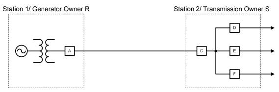
In Figure 2 above, the interconnecting Element between the Transmission to Generation Interconnected Facilities (Station 1 – Generation Owner R and Station 2 – Transmission Owner S) is the transmission line or bus between Breakers A and C.
