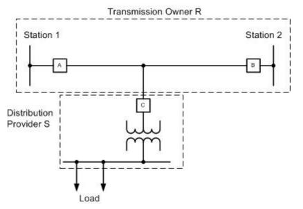
In Figure 4 above, the interconnecting Element between the Transmission Owner to Distribution Provider Interconnected Facilities (Transmission Owner R line between Breakers A and B – Distribution Provider S) is the transmission line or tap between the line and Breaker C.
