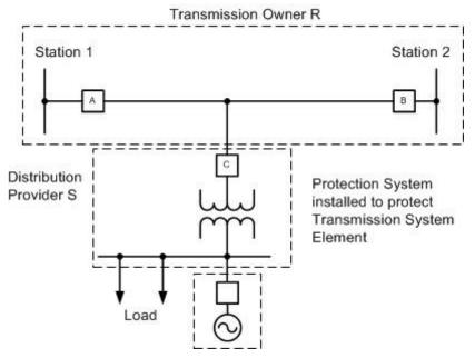
In Figure 3 above, the interconnecting Element between the Transmission Owner to Distribution Provider (with a generator) Interconnected Facilities (Transmission Owner R line between Breakers A and B – Distribution Provider S) is the transmission line or tap between the line and Breaker C.
