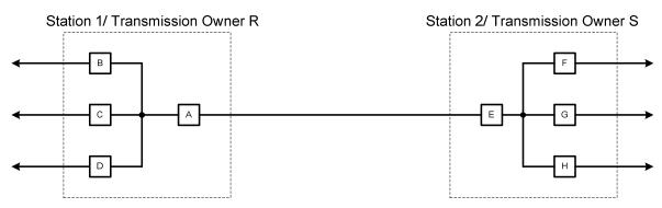
In Figure 1 above, the <u>I</u>interconnect<u>eding</u> Element between the Transmission <u>Owners</u> Interconnected Facilities (Station 1 – Transmission Owner R and Station 2 – Transmission Owner S)-is the transmission line between Breakers A and E.
