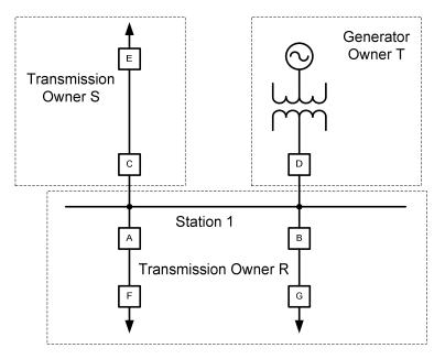
In Figure 5 above, the interconnecting Element between the Transmission Owners R and S and the Generation Owner T is the common Transmission bus. In this example, Transmission Owner S and Generator Owner T are not directly interconnected to each other at Transmission Station 1, and all direct interconnections are between Owner R and each of the other Owners connected to the bus.
