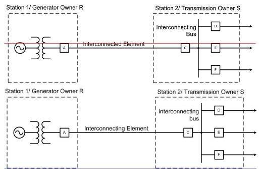
In Figure 2 above, the <u>InterconnectedInterconnecting</u> Element between the Transmission Owner and the Generator Owner is the transmission line or bus between Breakers A and C.
