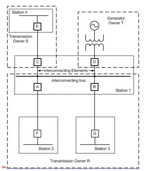
Figure 5 above, <u>illustrates</u> the <u>Interconnected ElementInterconnecting Elements</u> between the Transmission Owners R and S and Generator Owner T is the common Transmission bus. In this example, Transmission Owner S and Generator Owner T are not directly <u>interconnected interconnecting</u> to each other at Station 1. All direct interconnections are between
