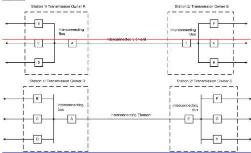
In Figure 1 above, the <u>InterconnectedInterconnecting</u> Element between the Transmission Owners is the transmission line between Breakers A and E.
