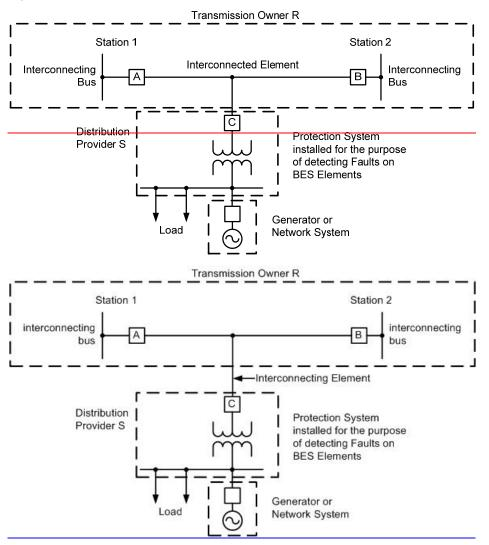
In Figure 3 above, the <u>InterconnectedInterconnecting</u> Element between the Transmission Owner and the Distribution Provider is the transmission line (or tap) between <u>the Distribution Provider's</u> Breaker C and the point of connection to the line between <u>the Transmission Owner's</u> Breakers A and B<u>. Therefore, the applicable Protection Systems per this standard are those at Breakers A, B and C.</u>
